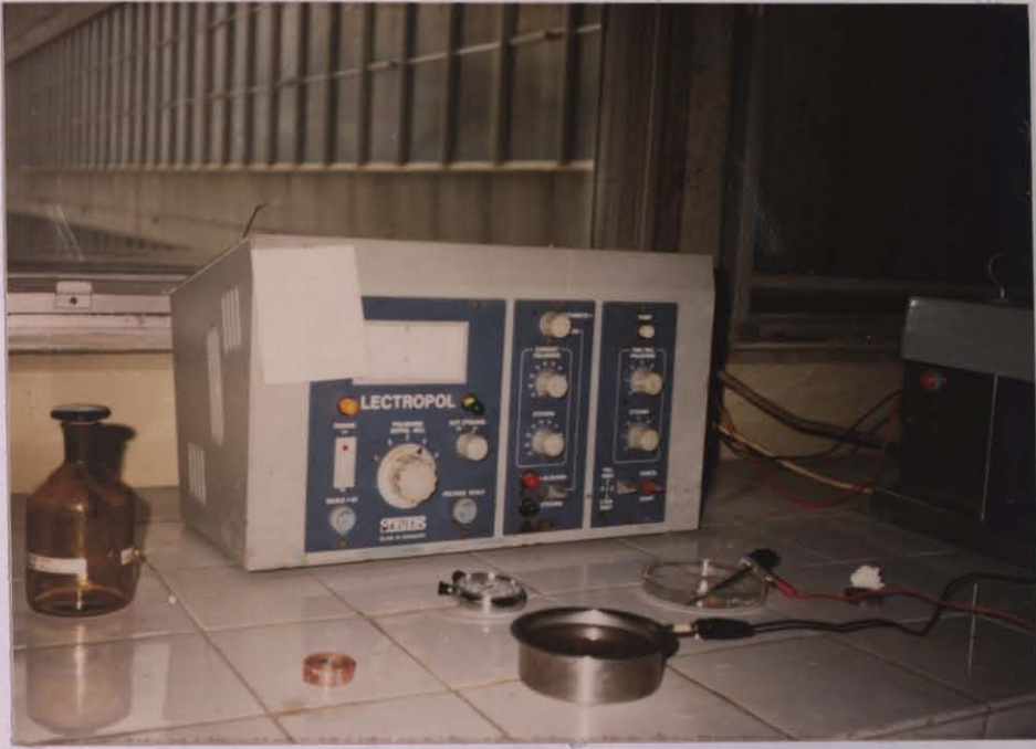
Figure 16 - Electrolytic Etching Apparatus.
