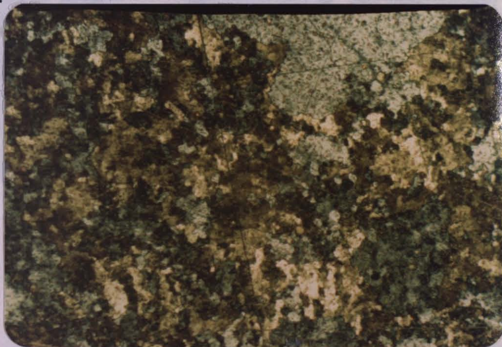
Figure 25 - Aluminum 1100, after hot-torsion at 250°C with a deformation rate of \dot{\gamma}^* = 6.84 \times 10^{-3} rad/s and cooling in air, polarized light, magnification 200 X.
