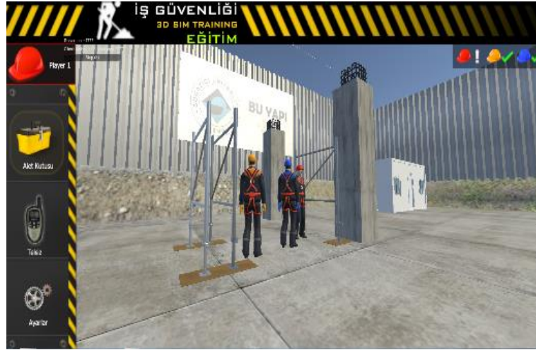
Figure 3.10. H Type Scaffoldings on the Adjustable Jacks.
