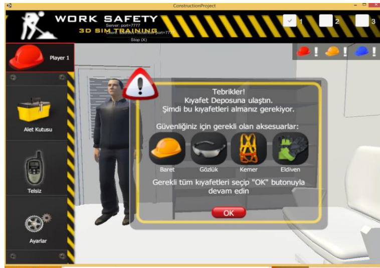
Figure 3.2. Personal Protection Equipment List in the Equipment Storage.
