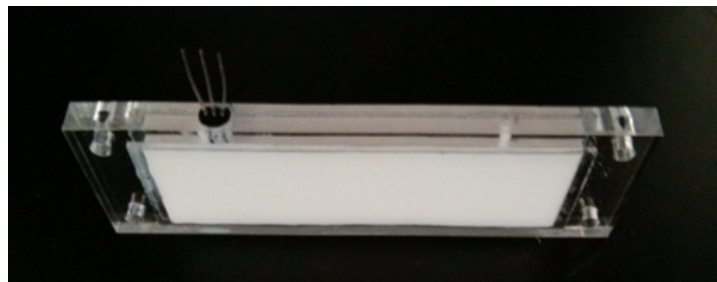
Figure 2.2 Sample cuvette with temperature sensor.
