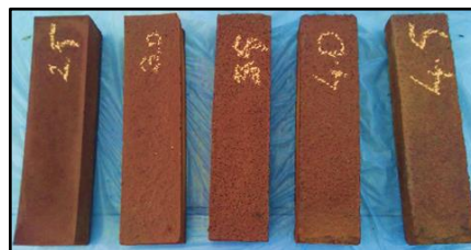
Figure 2.1. Images of synthesized volcanic ash based geopolymers
