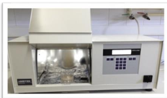
Figure 3.2. Solar irradiation initiated reactor configuration (Atlas Suntest CPS+).
