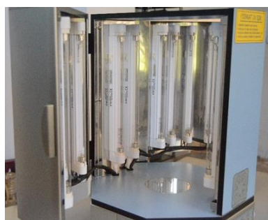
Figure 3.1. UVC irradiation initiated reactor configuration.
