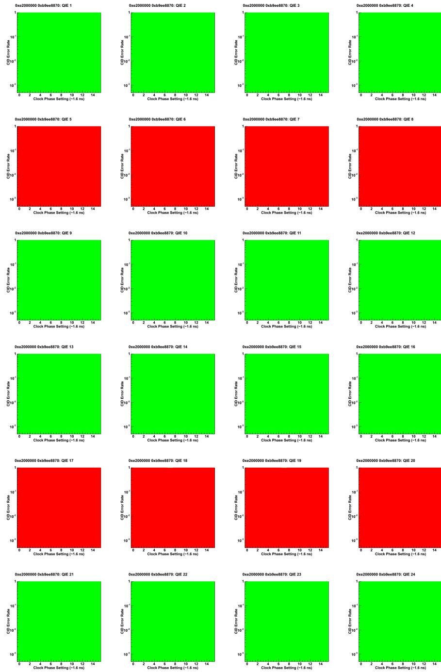
Figure 7.9. Result of a failed pedestal test due to the Igloo middle link issue. Middle link pattern can be seen on the 2nd and 5th rows.
