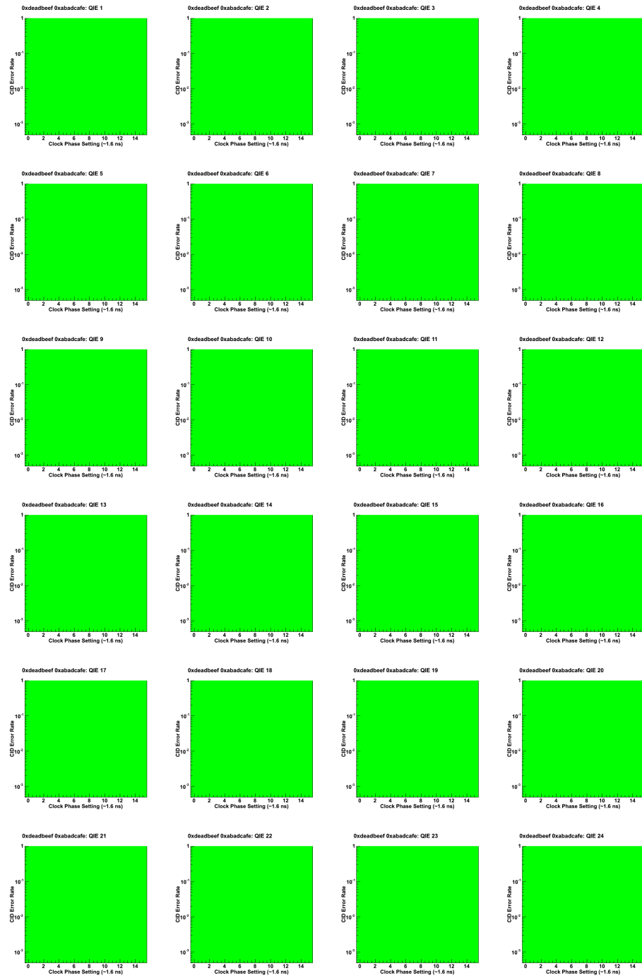
Figure 7.6. Result of a successful Cap ID test. Each histogram corresponds to one QIE chip. The horizontal axis of each histogram represents the clock phase setting. Each row of histograms represents an Igloo2 link.
