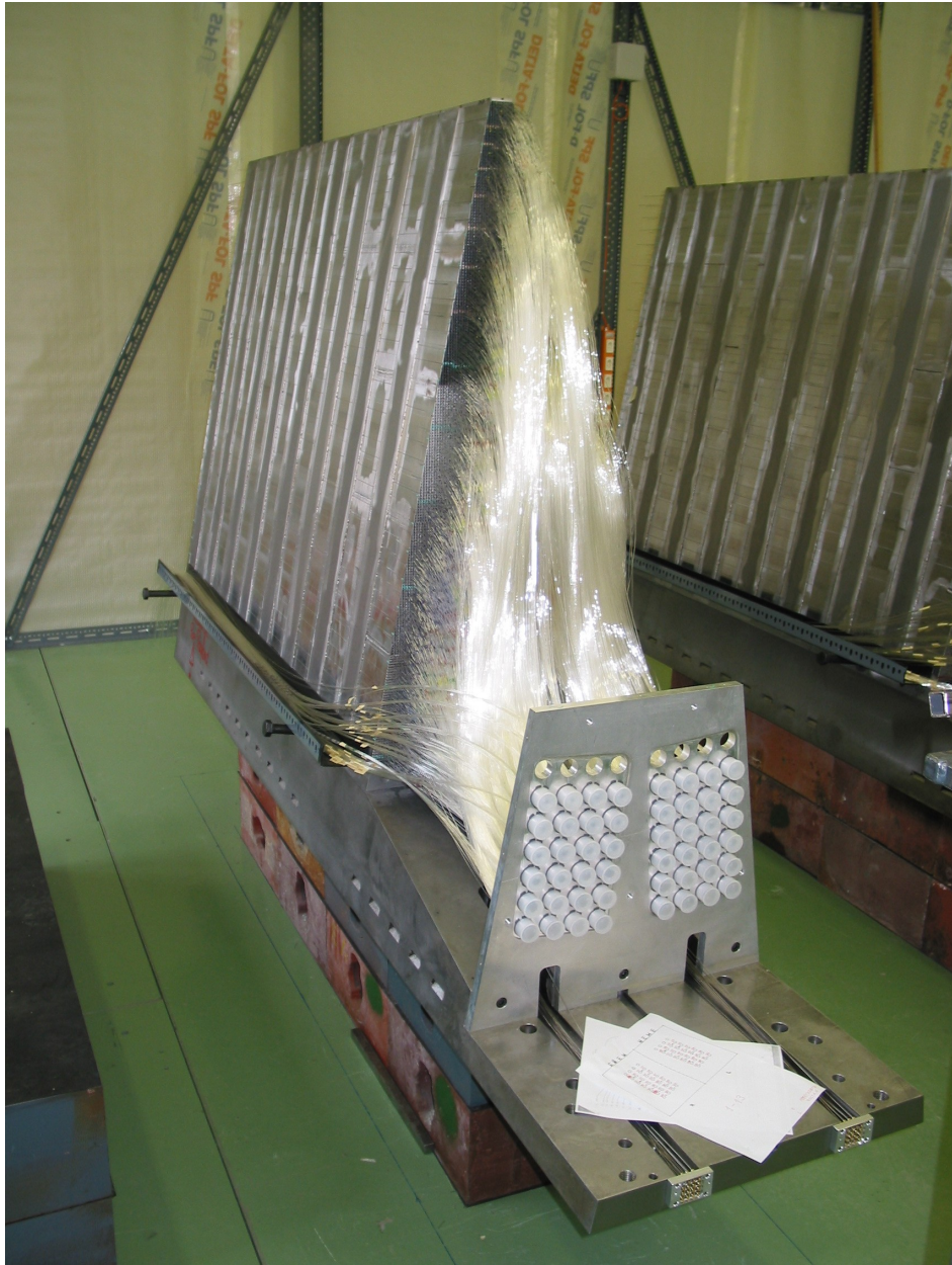
Figure 5.2. One of the steel wedges of the HF with its quartz fibers attached. Mounting slots for ROBOXs can also be seen. [10]
