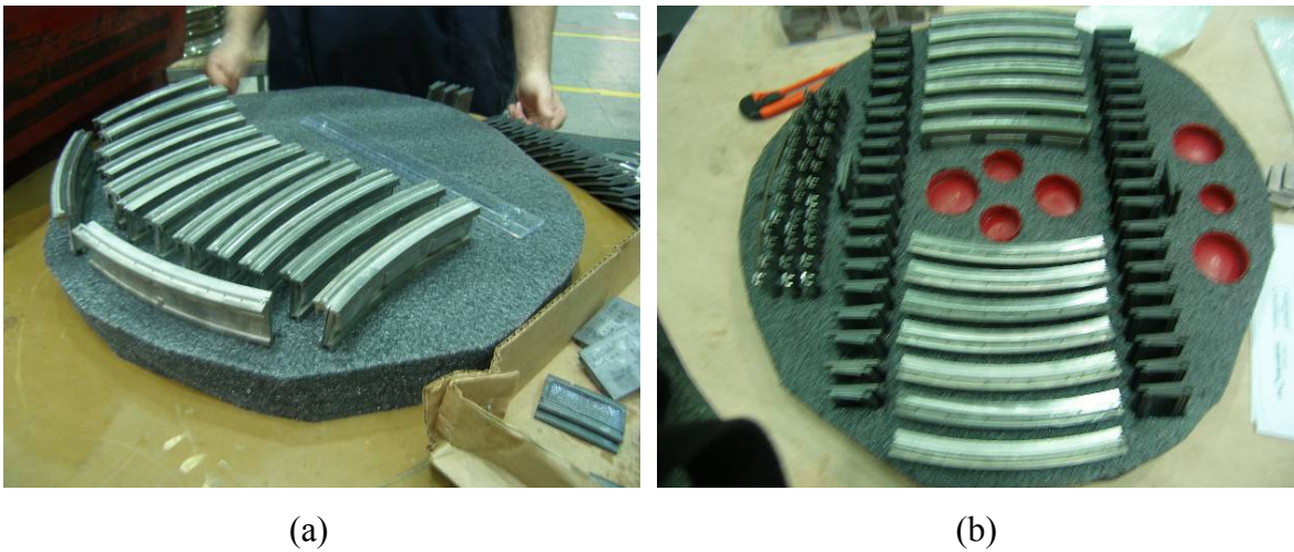
Figure 5.46. Technician designing the part kit for his ease of use (a) and final part kit (b)
