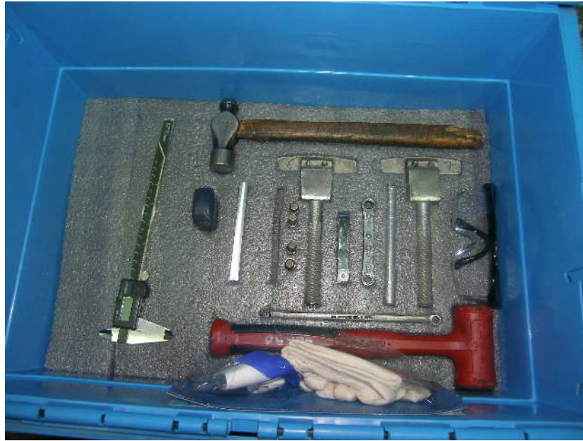
Figure 5.30. Tool kit for HPC forward case assembly
