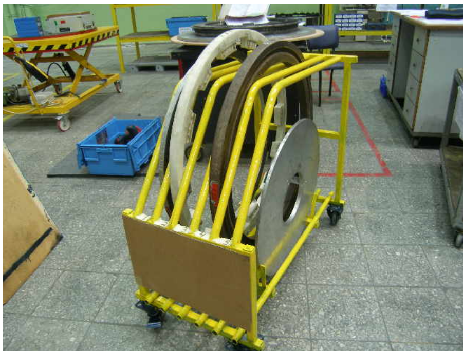
Figure 5.48. Special tool cart for HPT shroud and LPT nozzle assembly
