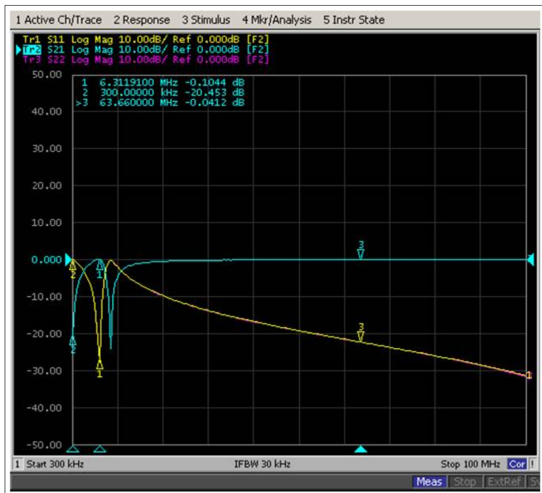
Figure 3.29 S21 measurements of leakage block circuit using 1000 pF capacitors at 63.66 MHz and 300 kHz.
