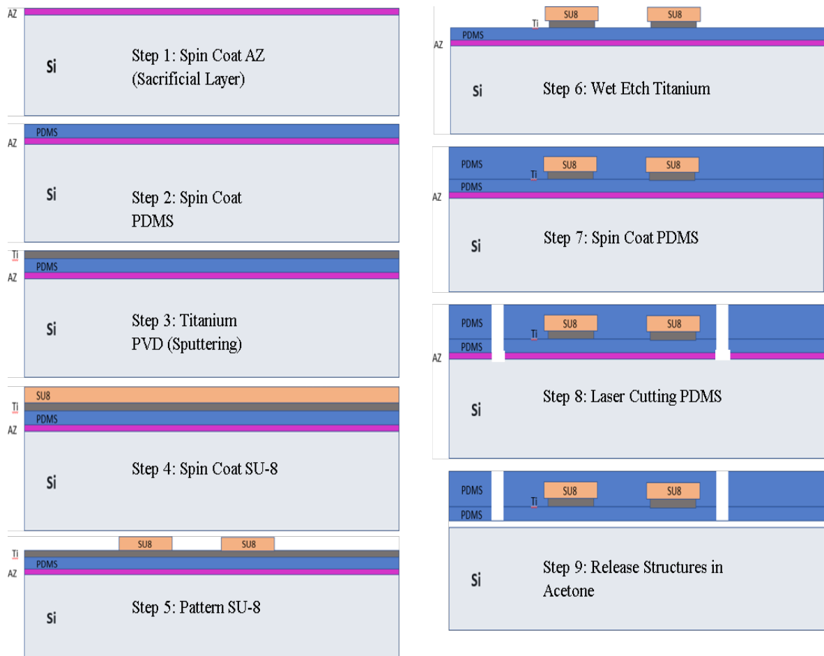
Figure 2.13. SRR embedded in PDMS fabrication process flow.
