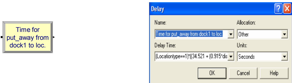
Figure 4.19. Delay module for determining put away time of products from dock1 to locations
