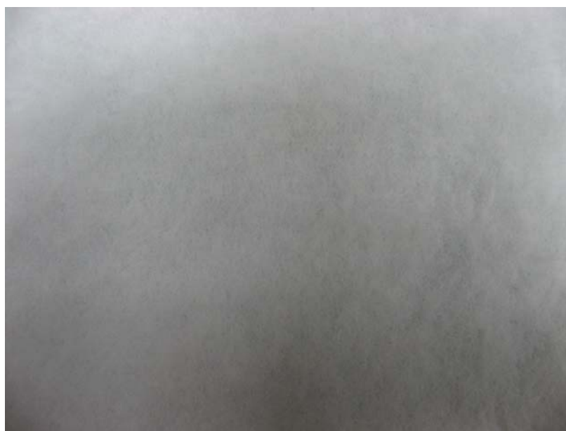
Figure 3.19. Polypropylene, staple fiber, needlepunched nonwoven geotextile (N1)
