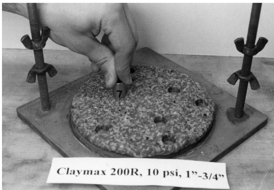
Figure 2.44. Sampling water content and bentonite mass per area of a GCL-1 specimen (Fox et al., 2000)
