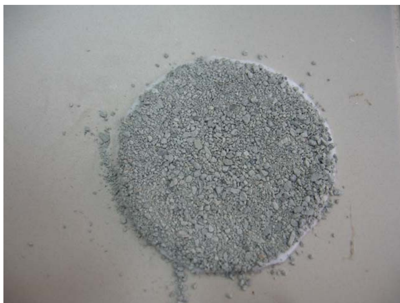
Figure 3.29. Granular bentonite placed over a nonwoven geotextile
