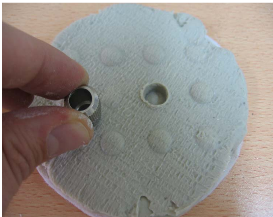
Figure 3.43. Sampling mass per unit area and moisture content of a GCL-2 sample after termination of a flexible wall triaxial permeability test
