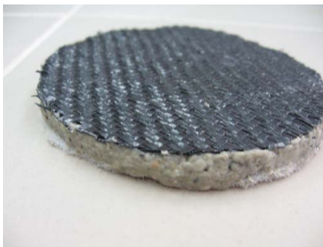
Figure 3.31. GCL-4 specimen where sodium bentonite is sandwiched between woven geotextile (W2) and nonwoven geotextile (N1)
