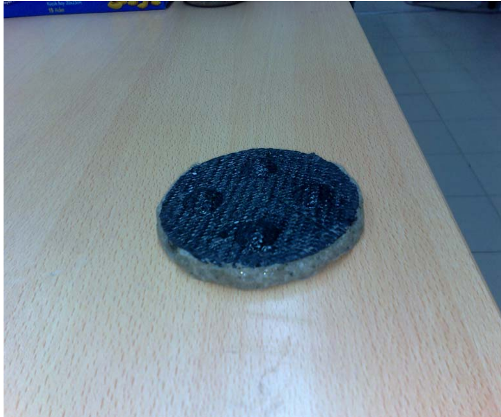
Figure 4.69. GCL-4-W-D2 sample after the termination of the flexible wall triaxial permeability test
