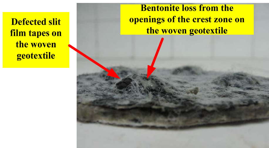
Figure 4.11. GCL-1-W-D2 sample after the termination of the flexible wall triaxial permeability test
