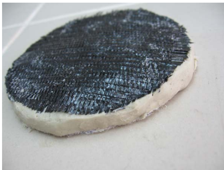
Figure 3.33. GCL-3 specimen where calcium bentonite is sandwiched between woven geotextile (W1) and nonwoven geotextile (N1)
