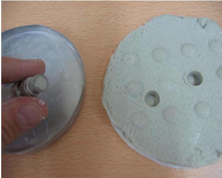
Figure 3.45. A sampling tube with bentonite inside placed in a can
