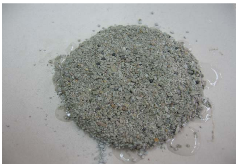
Figure 3.30. Soaked bentonite on a nonwoven geotextile
