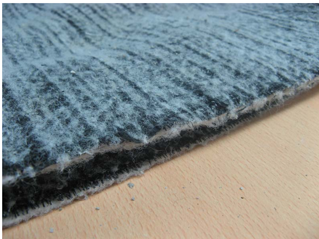
Figure 3.17. Woven geotextile component of Bentomat SS100 (GCL-1)
