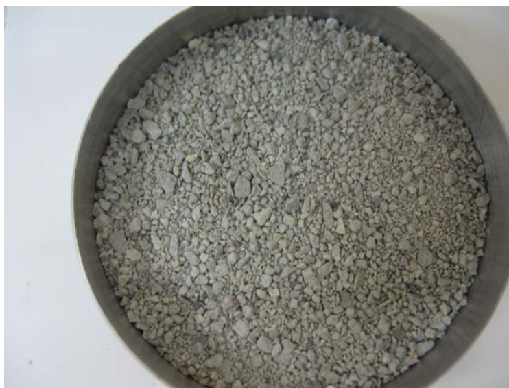
Figure 3.22. Granular sodium bentonite used in GCL-1 (SB)
