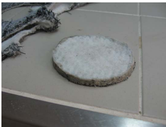
Figure 3.28. GCL-1 specimen where the nonwoven geotextile is on the top
