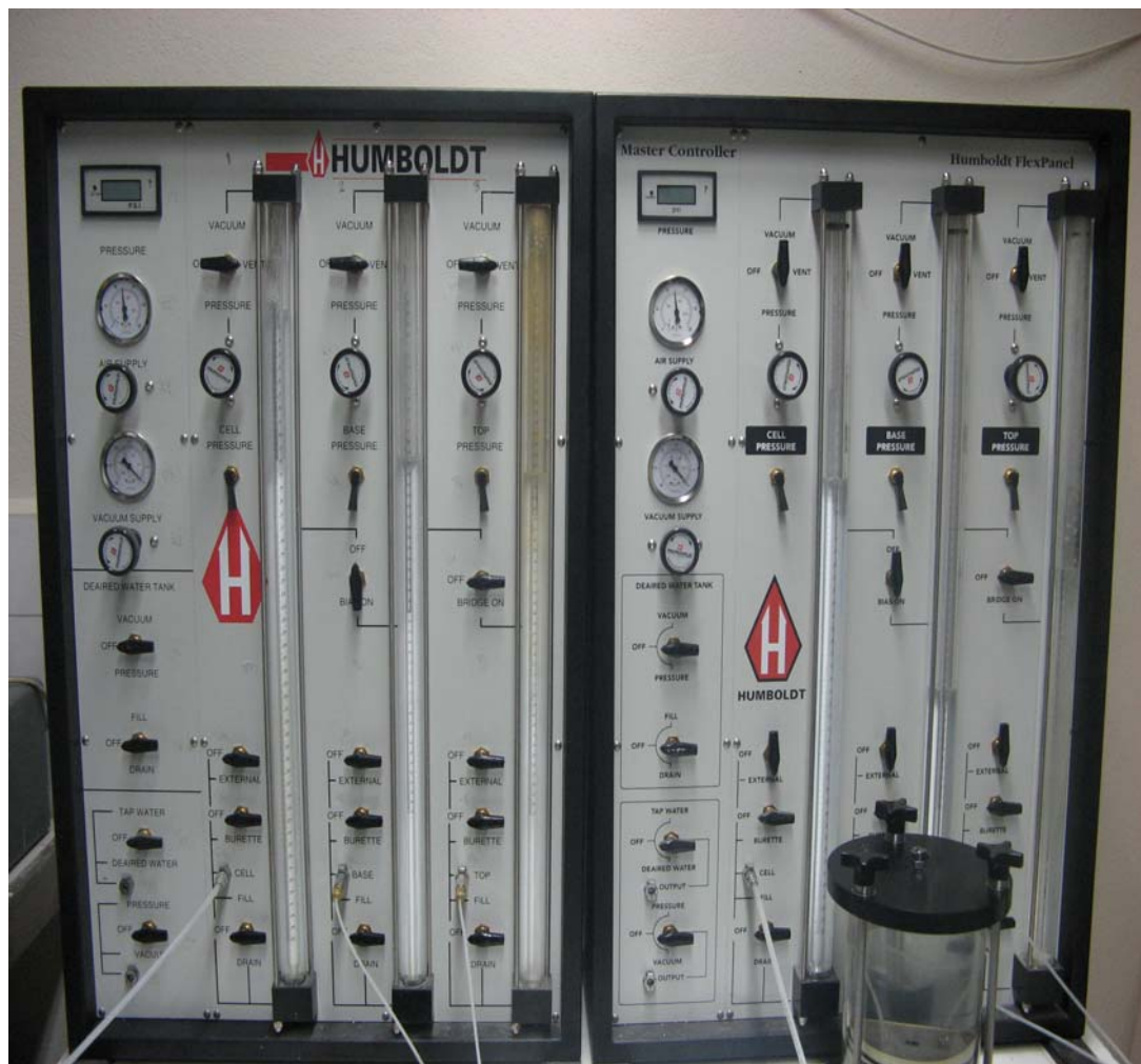
Figure 3.1. HM-4150 Flexpanels for Triaxial Permeability Tests
