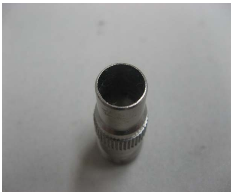
Figure 3.44. Sampling tube made of thin-walled steel cylinder having 7.5 mm diameter and 23 mm height for mass per unit area and moisture content determination of the bentonite
