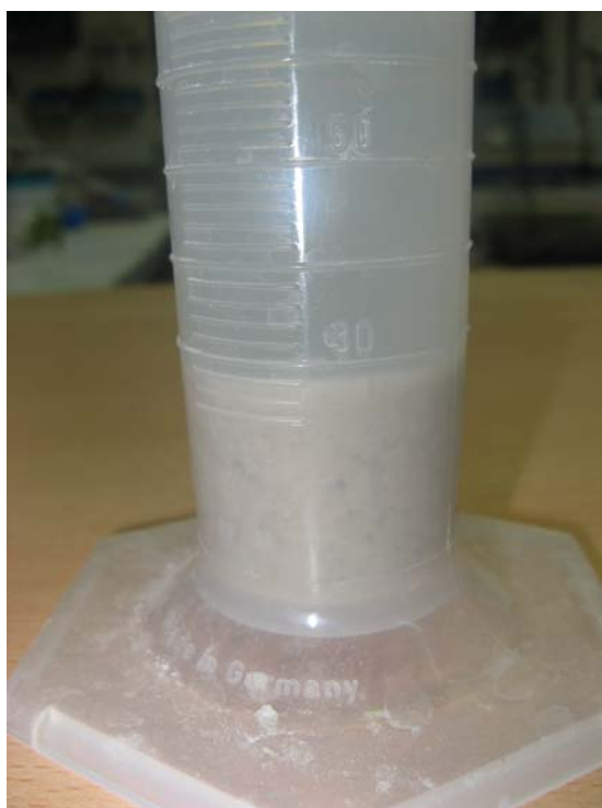
Figure 3.23. Swell Index test result for sodium bentonite (SB) in a graduated cylinder
