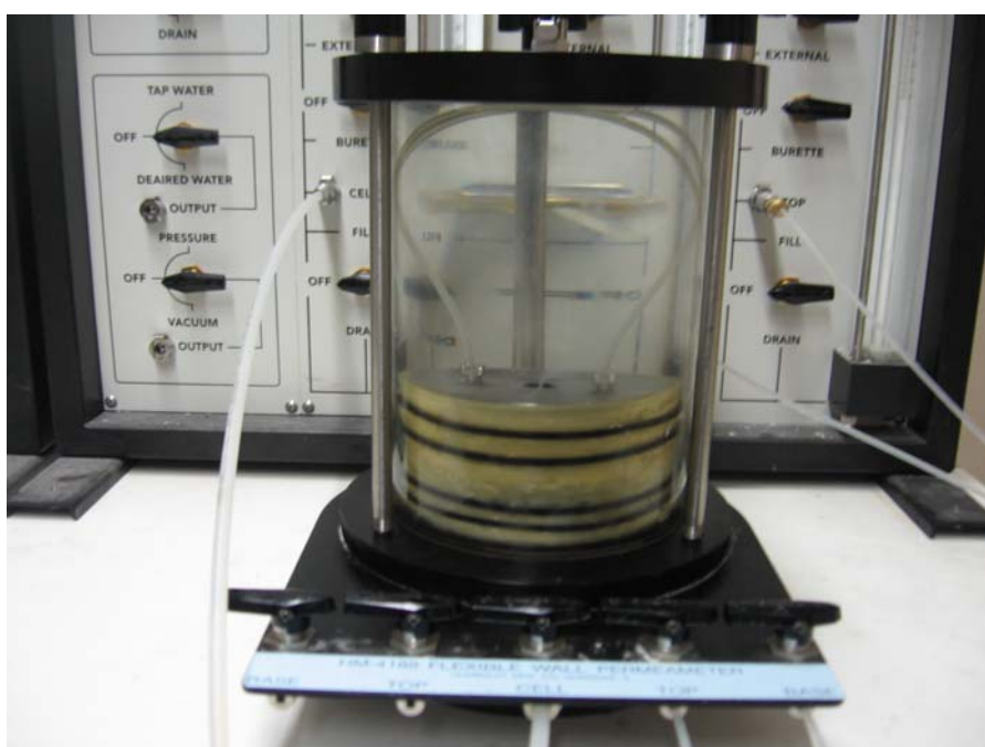
Figure 3.42. GCL sample covered with latex membrane and O-rings in flexible wall triaxial permeameter cell
