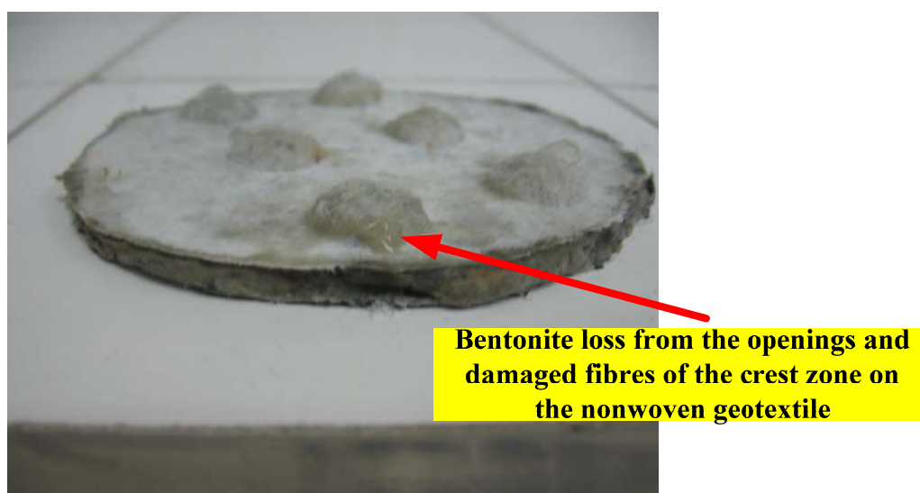
Figure 4.32. GCL-2-NW-D1.5 sample after the termination of the flexible wall triaxial permeability test
