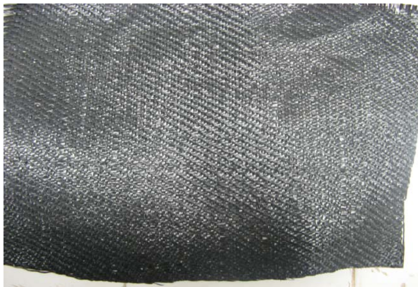
Figure 3.21. Polypropylene woven geotextile (W2)
