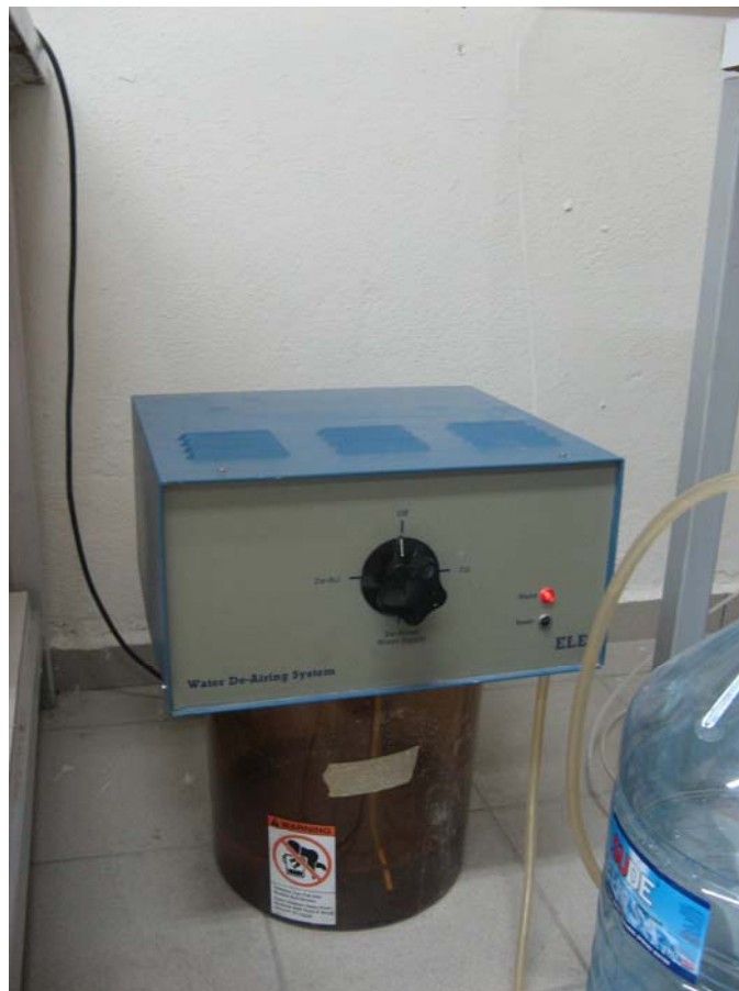
Figure 3.3. De-aired water supplier
