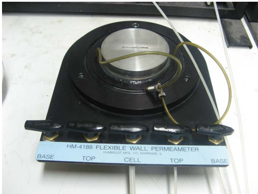
Figure 3.5. Base pedestal of the permeameter cell
