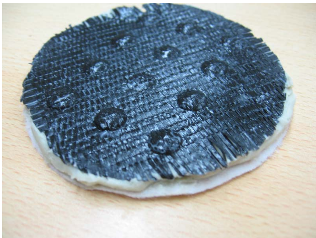
Figure 4.64. GCL-3-W-D1 sample after the termination of the flexible wall triaxial permeability test
