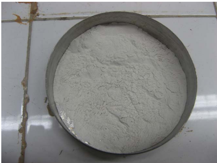
Figure 3.24. Powdered calcium bentonite used in GCL-3 (CB)
