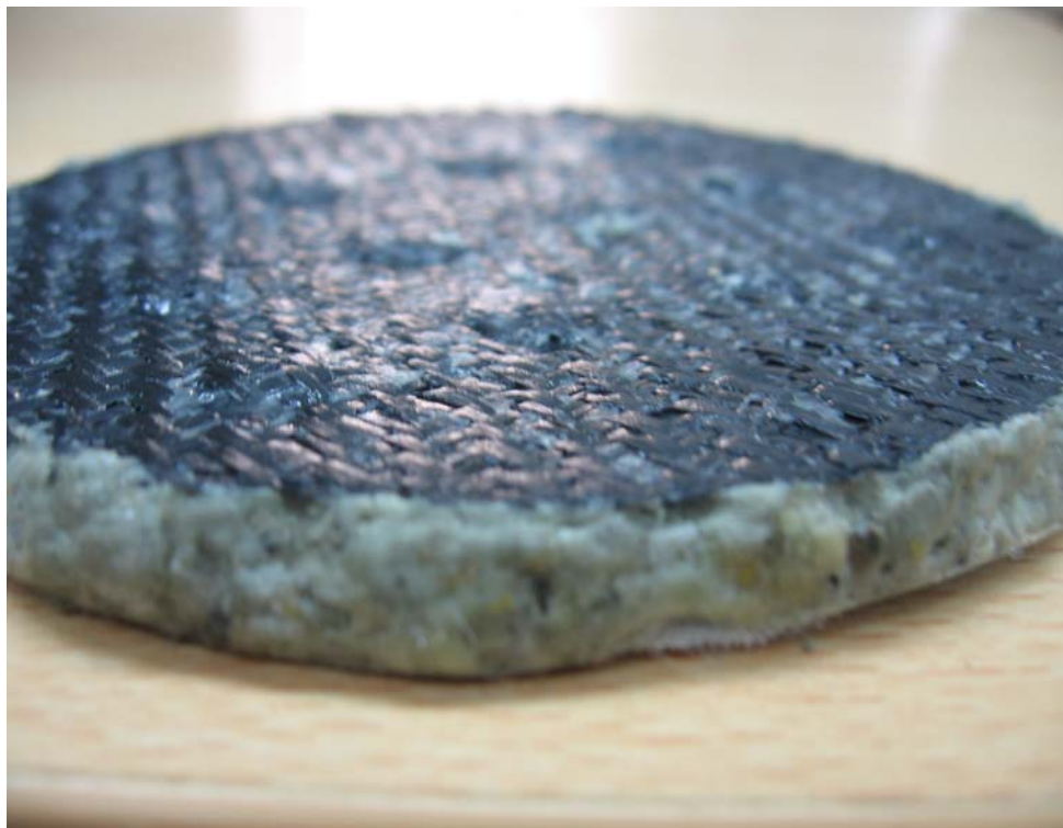
Figure 4.75. GCL-4-W-D1 sample after the termination of the flexible wall triaxial permeability test
