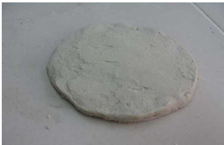
Figure 3.32. Soaked calcium bentonite placed on a nonwoven geotextile
