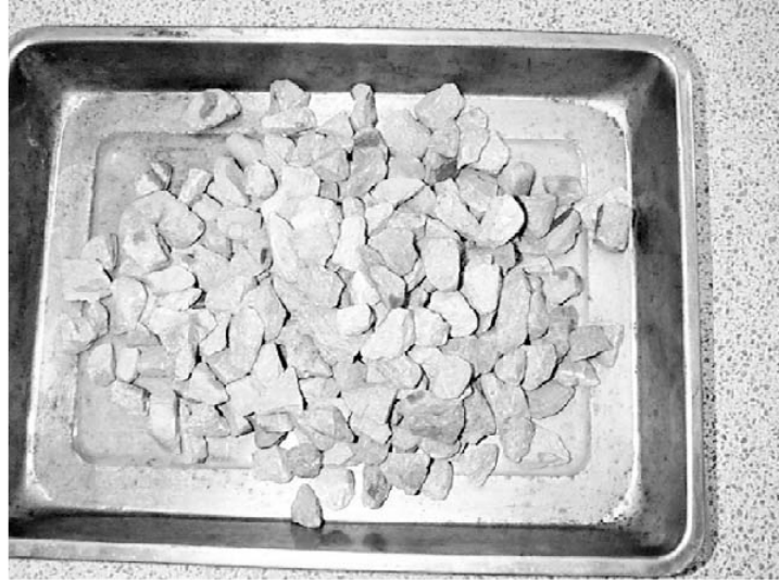
Figure 2.53. Crushed stone with diameter ranging from 25.4 mm to 50.8 mm (Shan and Chen, 2003)
