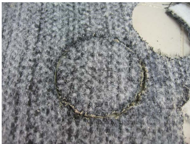
Figure 3.26. GCL specimen with its soaked perimeter during cutting process
