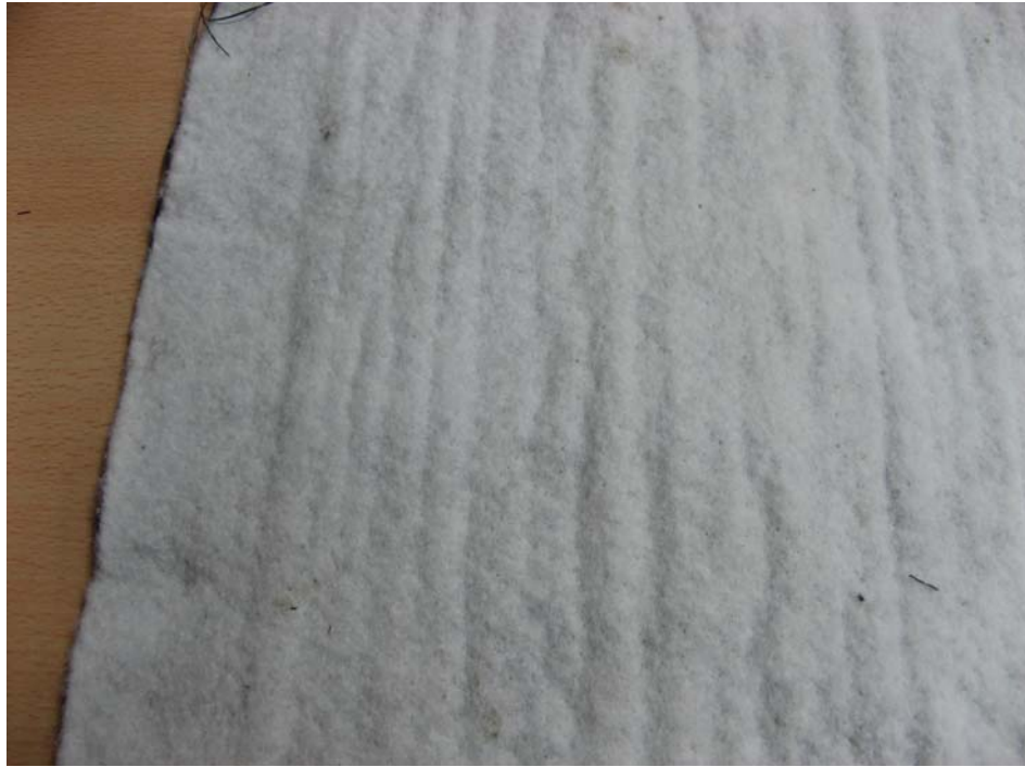
Figure 3.18. Nonwoven geotextile component of Bentomat SS100 (GCL-1)
