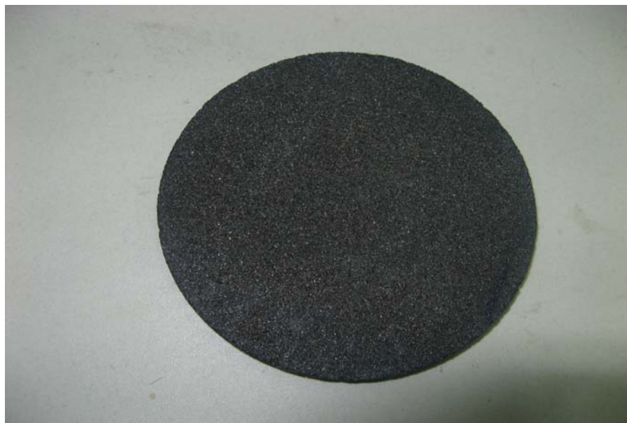
Figure 3.6. Porous stone used in the permeameter cell
