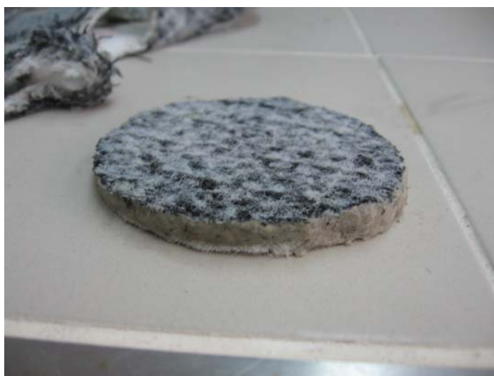
Figure 3.27. GCL-1 specimen where the woven geotextile is on the top
