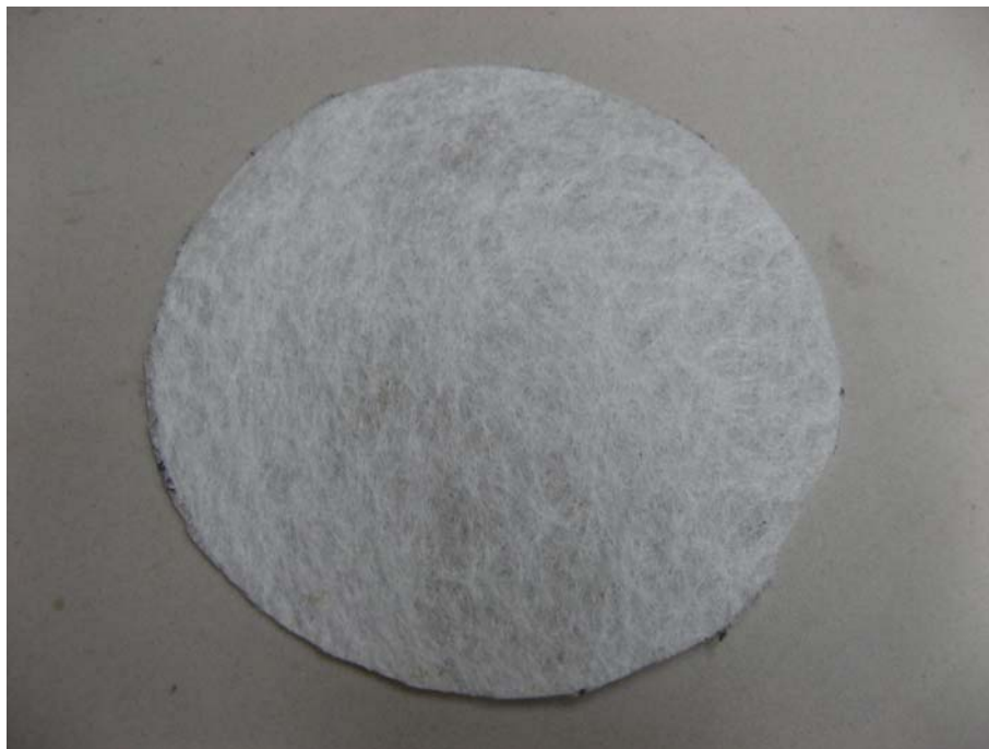
Figure 3.8. Nonwoven geotextile 120 NW used instead of filter paper
