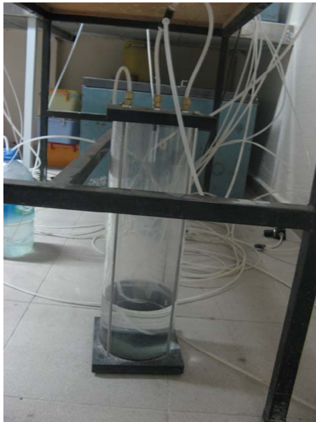
Figure 3.2. De-aired water tank
