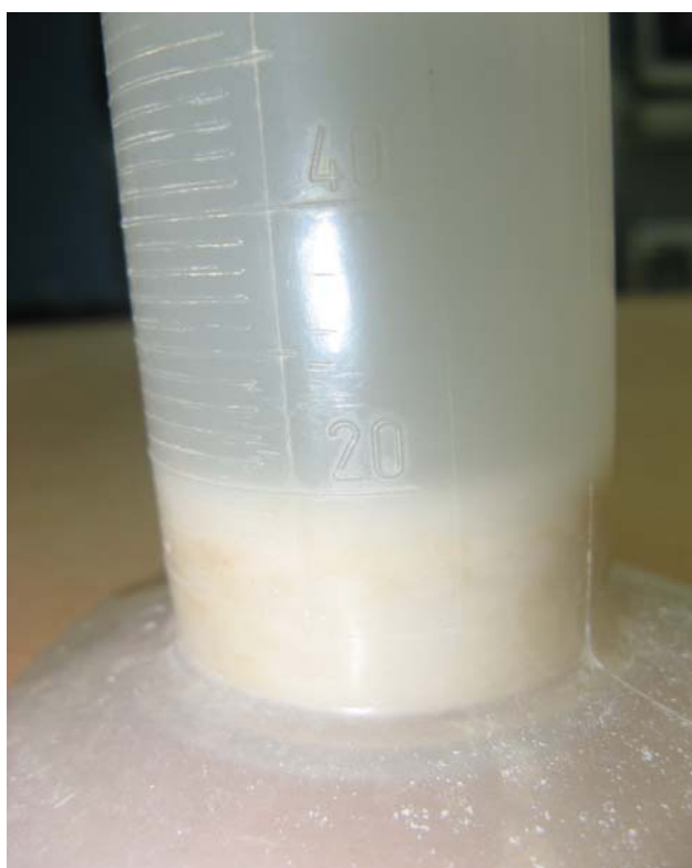
Figure 3.25. Swell Index test result for calcium bentonite (CB) in a graduated cylinder
