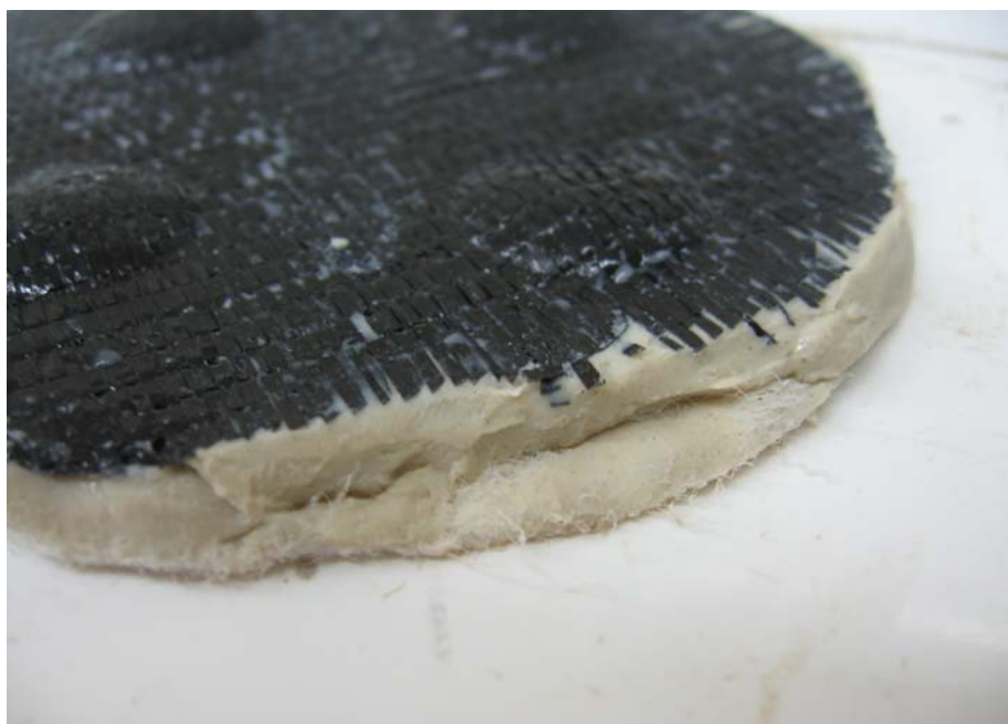
Figure 4.54. GCL-3-W-D2 sample after the termination of the flexible wall triaxial permeability test
