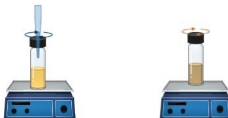
Figure 3.1 Seed solution was prepared by using a hot plate stirrer with the stock solutions of CTAB and HAuCl_4 and fresh solution of NaBH_4 .
