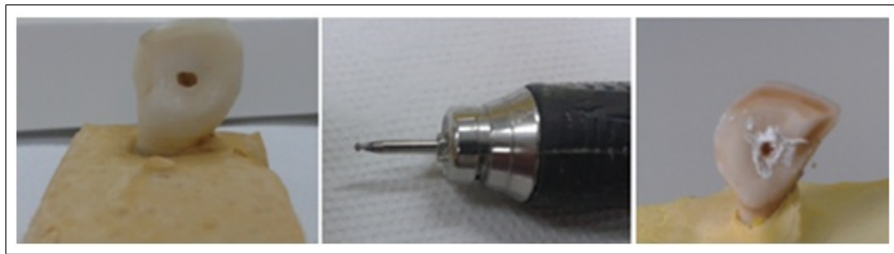
Figure 3.7 Drilled lingual surface of teeth, a round bur and silicon thermal paste filled cavity.
