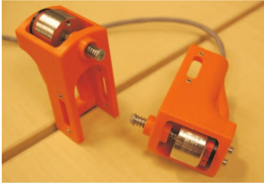
Figure 2.1. Voice coil motors used for surgical robot in [46].
