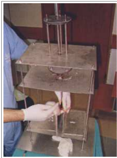
Figure 2.6 Creation of closed fracture by the Guillotine system
