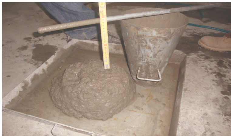
Figure 3.5. Determination of the slump on fresh concrete.
