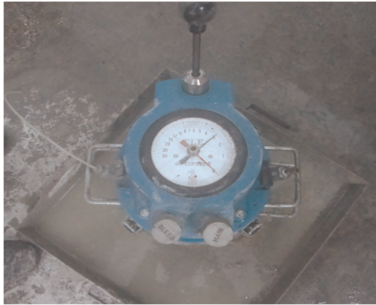
Figure 3.6. Determination of air content on fresh concrete.
