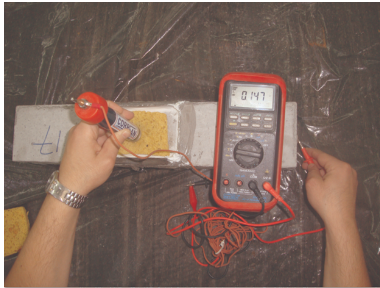
Figure 3.12. Half-Cell potential measurement.
