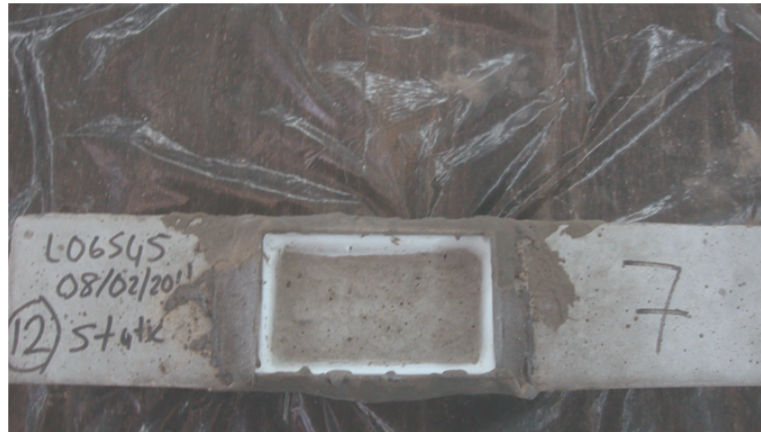
Figure 3.10. Reservoir on concrete surface.
