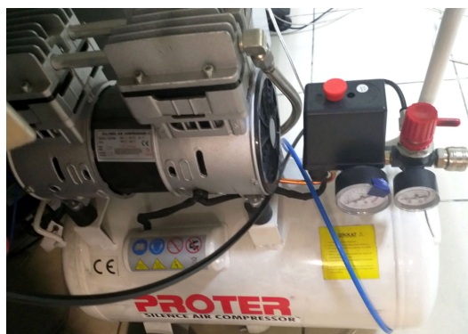
Figure 4.23. Pressurized tank with compressor that is used as the main pressure source.
