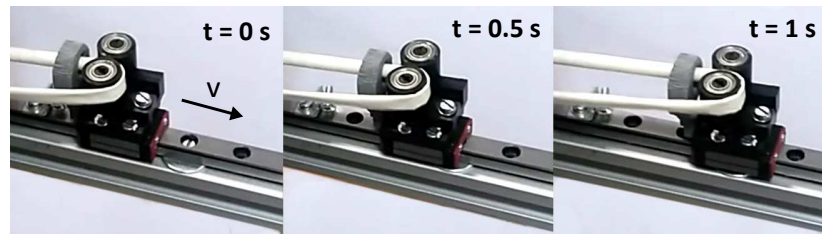
Figure 3.7. The actuator extending at constant speed while the slack section is released by the motor. Composite PA12/L tubing with 5 mm OD is used.
