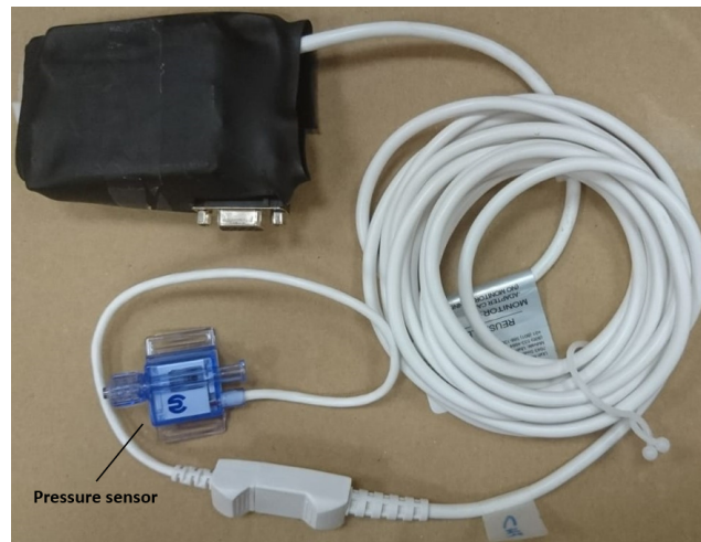
Figure 4.3. The pressure sensor which was placed to the patient corpus cavernosum to measure the ICP during the phases of erection
