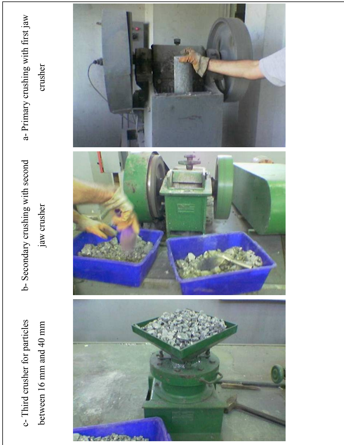
Figure A.1. Recycled aggregate production stages
