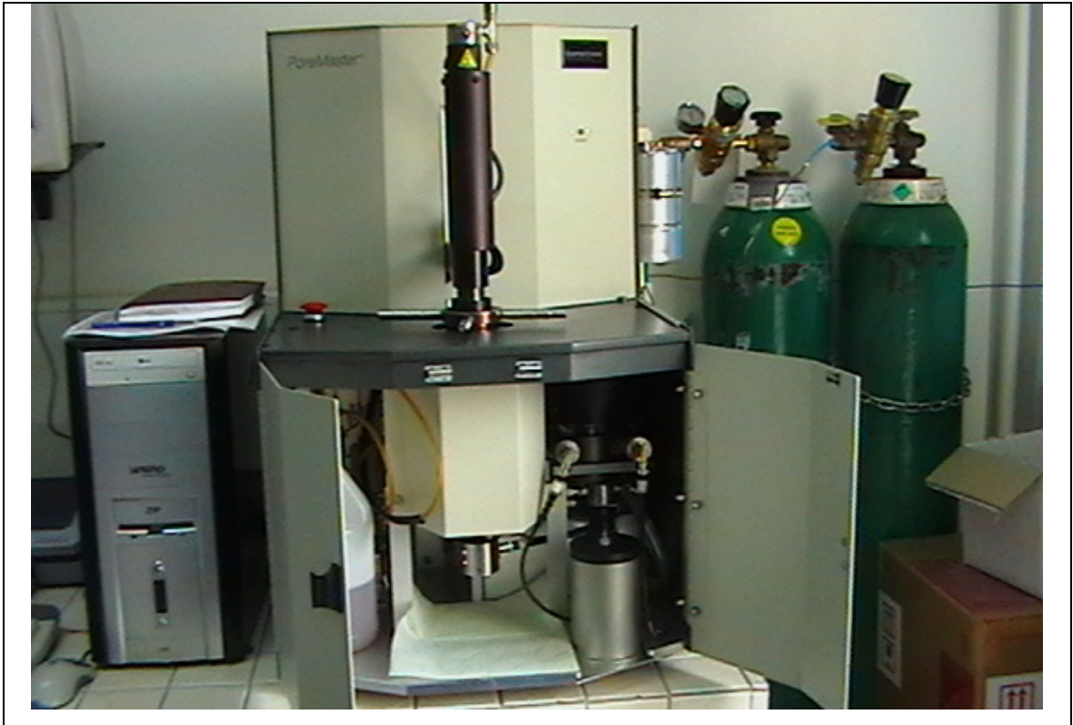
Figure 4.13. Quantachrome Poremaster equipment for MIP
