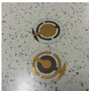
Figure 2.8 Cr/Au QCM Crystals.
