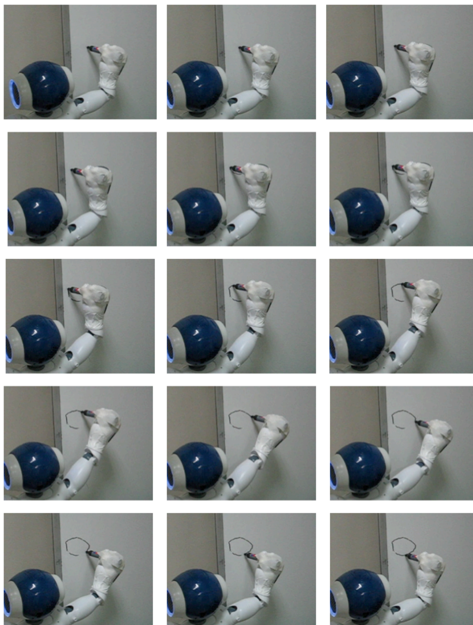
Figure 4.25. Robot drawing a circle.
