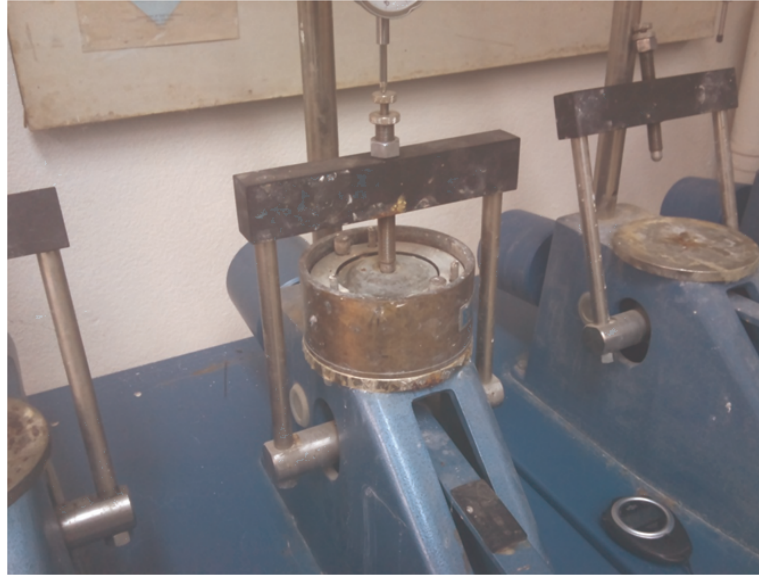
Figure 3.11. Constrained modulus test.
