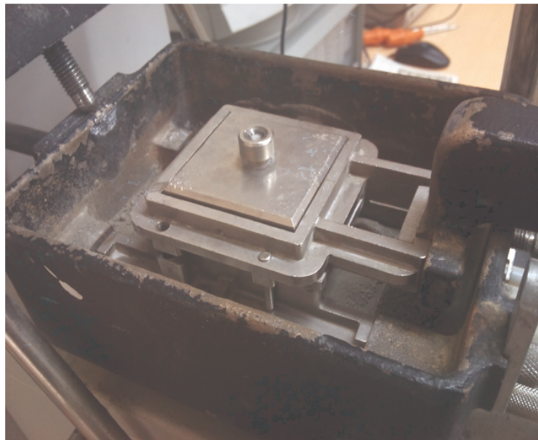
Figure 3.12. Direct shear box with dimensions of 60x60x28 mm.
