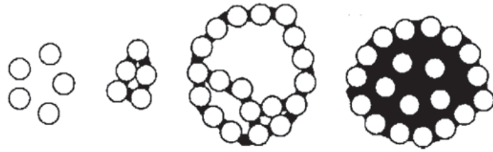
Figure 2.6. Mechanism of ball nuclei formation (water content below optimum state) (Yukio et al. , 1999).
