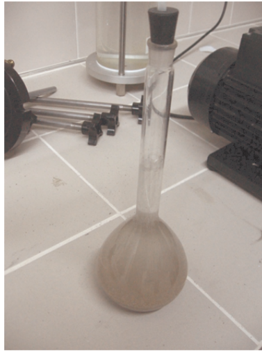
Figure 3.6. Specific Gravity Experiment Setup.
