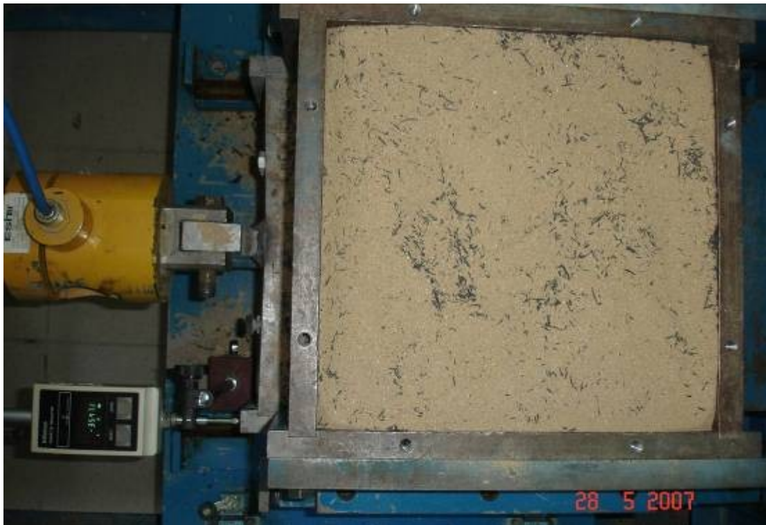
Figure 5.39. 10 per cent TB1 placed in the shear box
