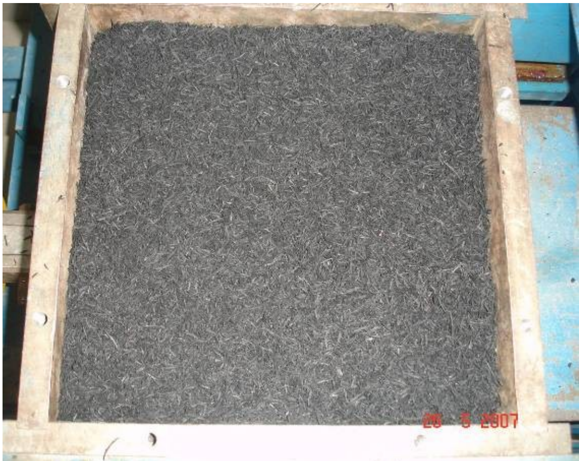
Figure 5.24. 100 per cent TB1 placed in the shear box
