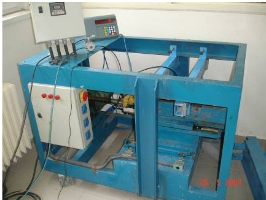
Figure 4.12. Large scale direct shear test apparatus
