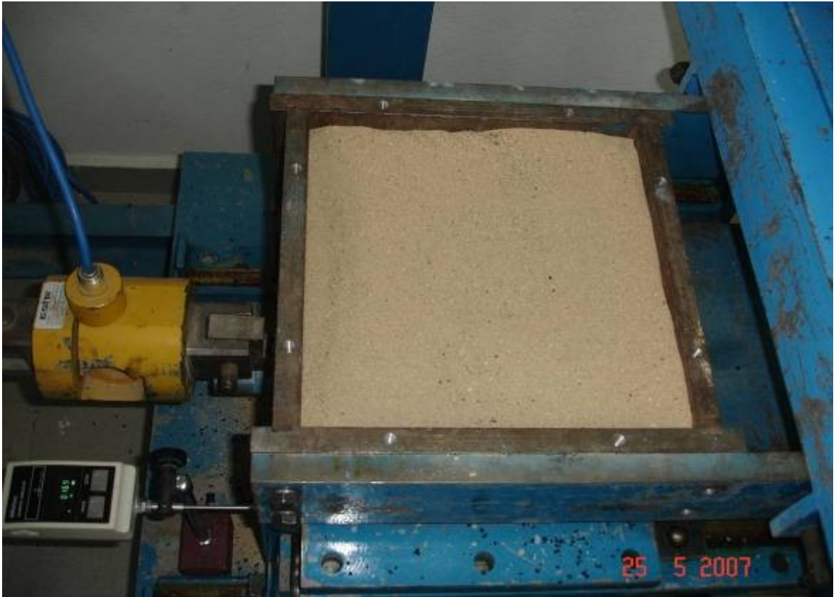
Figure 5.17. Sand Sample placed in the shear box
