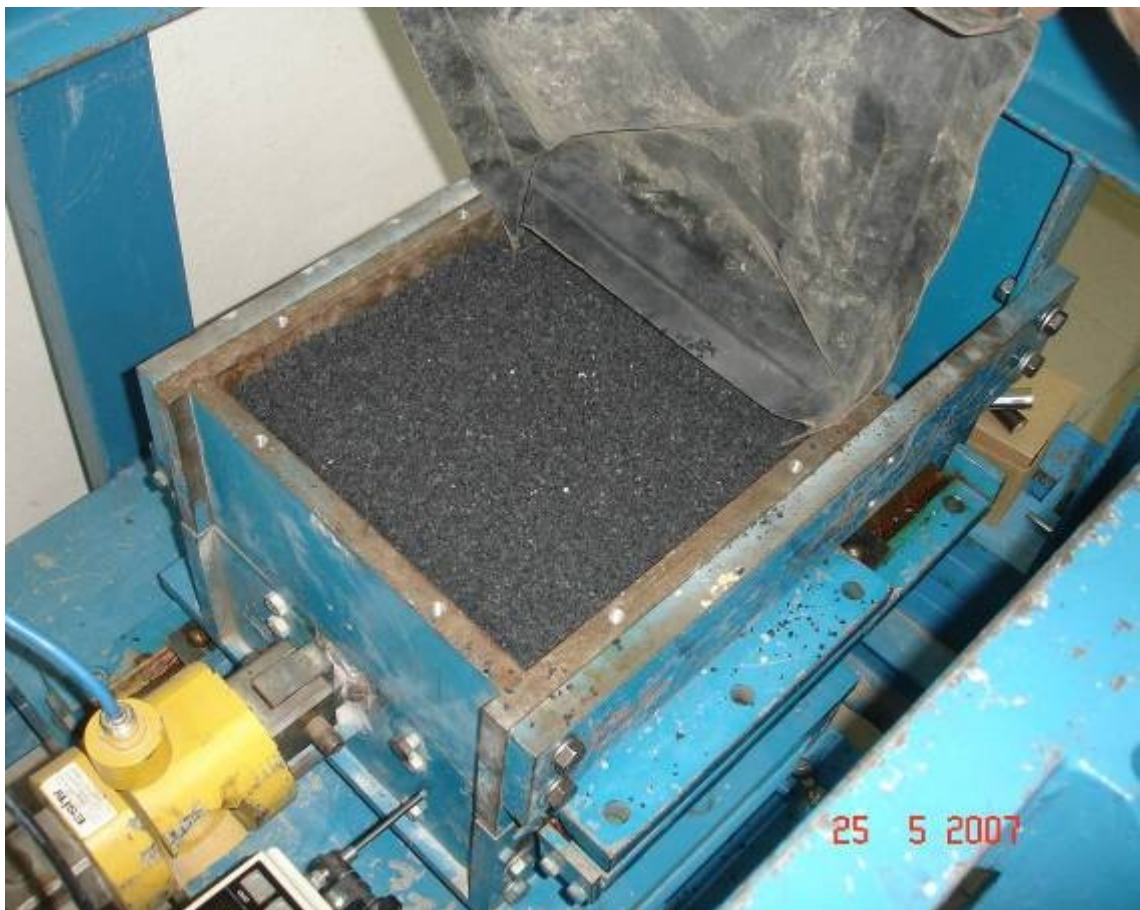
Figure 5.21. 100 per cent Tire crumb placed in the shear box
