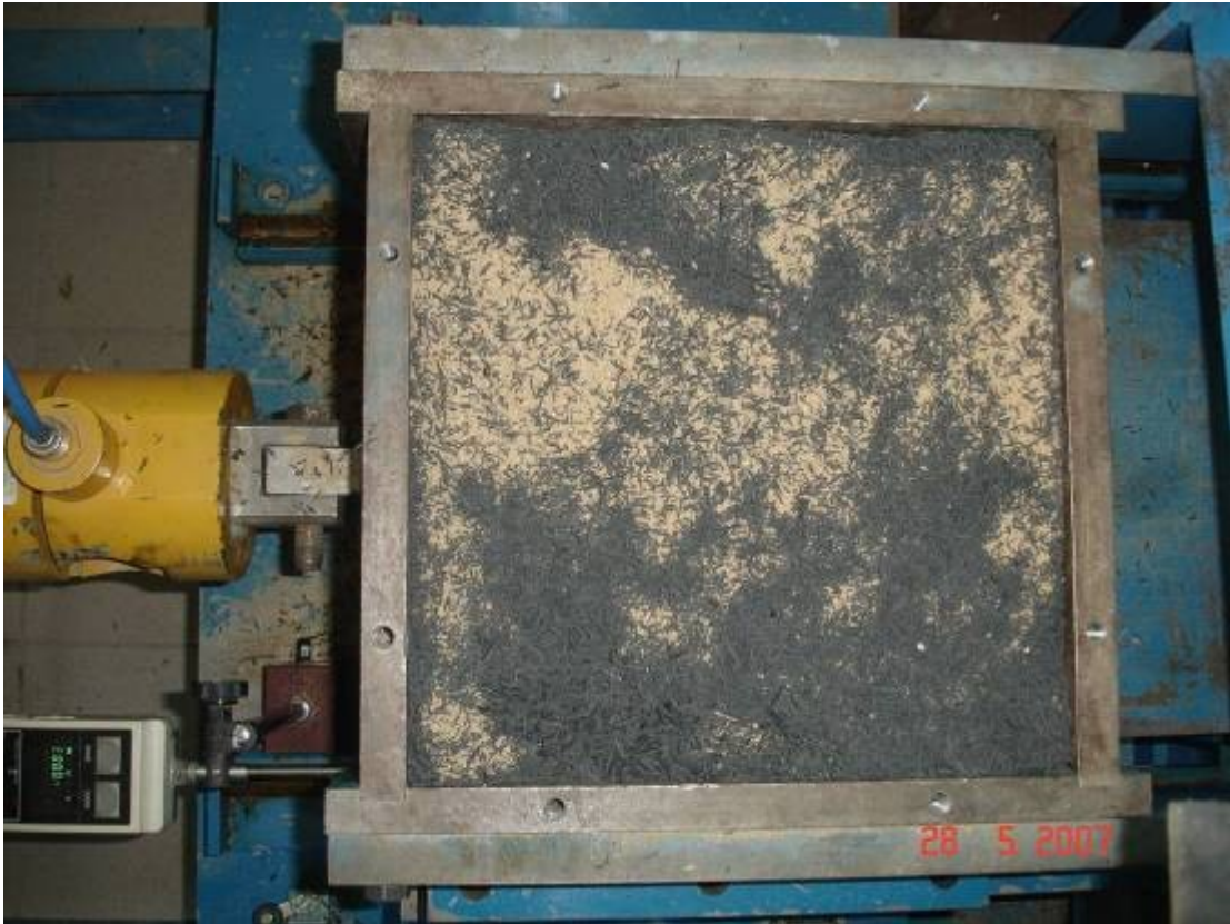
Figure 5.43. 20 per cent TB1 placed in the shear box
