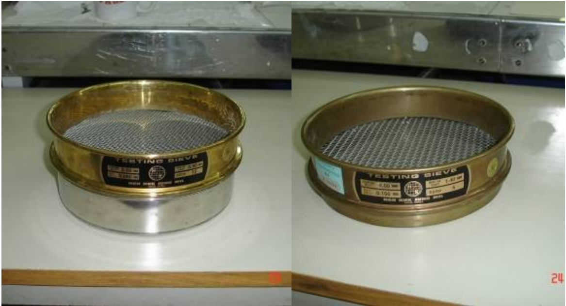
Figure 4.5. Sieves used to grade the tire buffings; 2mm and 4mm respectively
