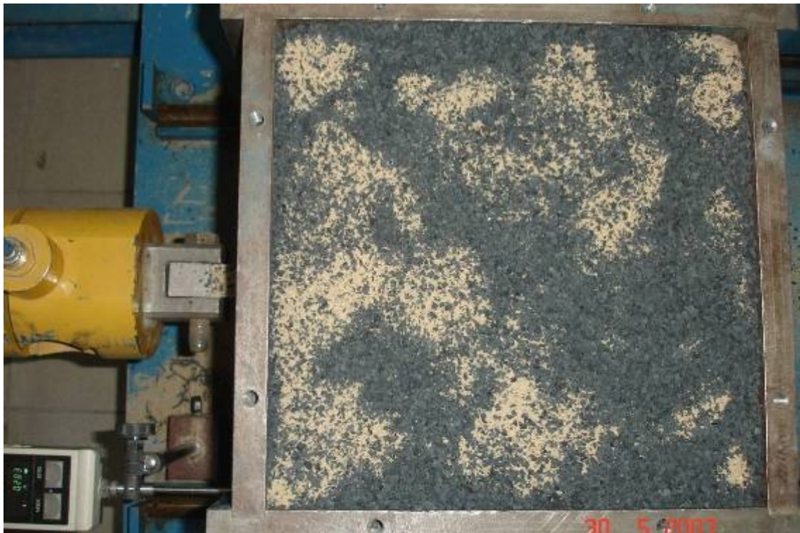
Figure 5.36. 30 per cent Tire crumb placed in the shear box
