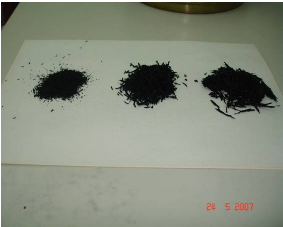
Figure 4.4. Graded tire buffings; dust, TB1 (2mm-4mm), TB2(>4mm) respectively.
