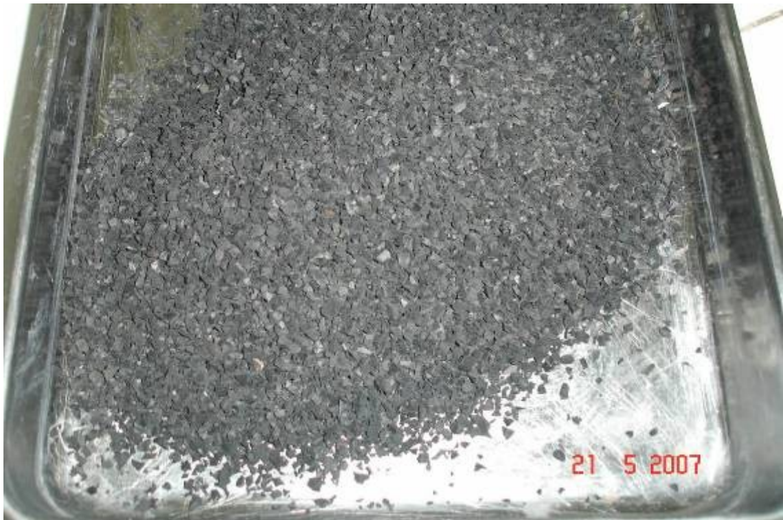
Figure 4.3. Tire crumb sample
