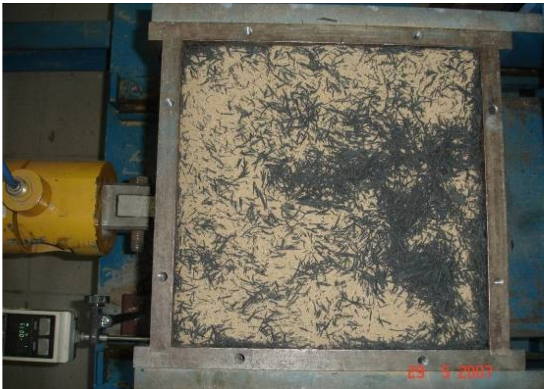
Figure 5.50. 10 per cent TB2 placed in the shear box
