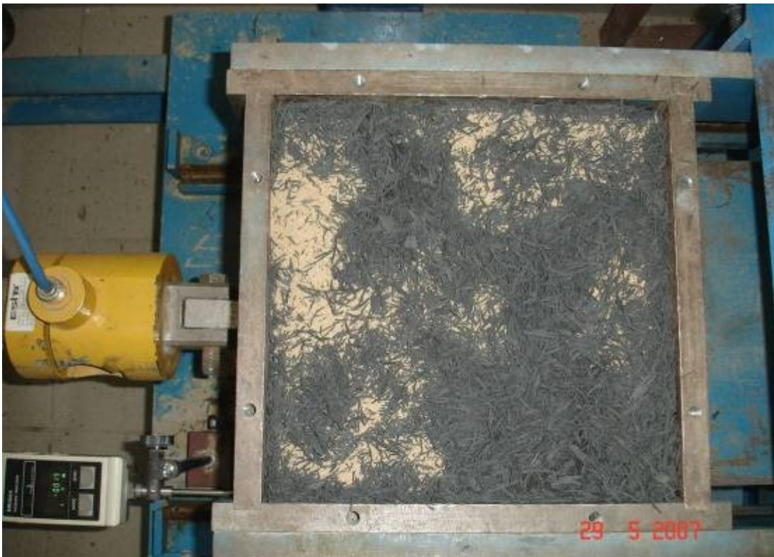
Figure 5.54. 20 per cent TB2 placed in the shear box
