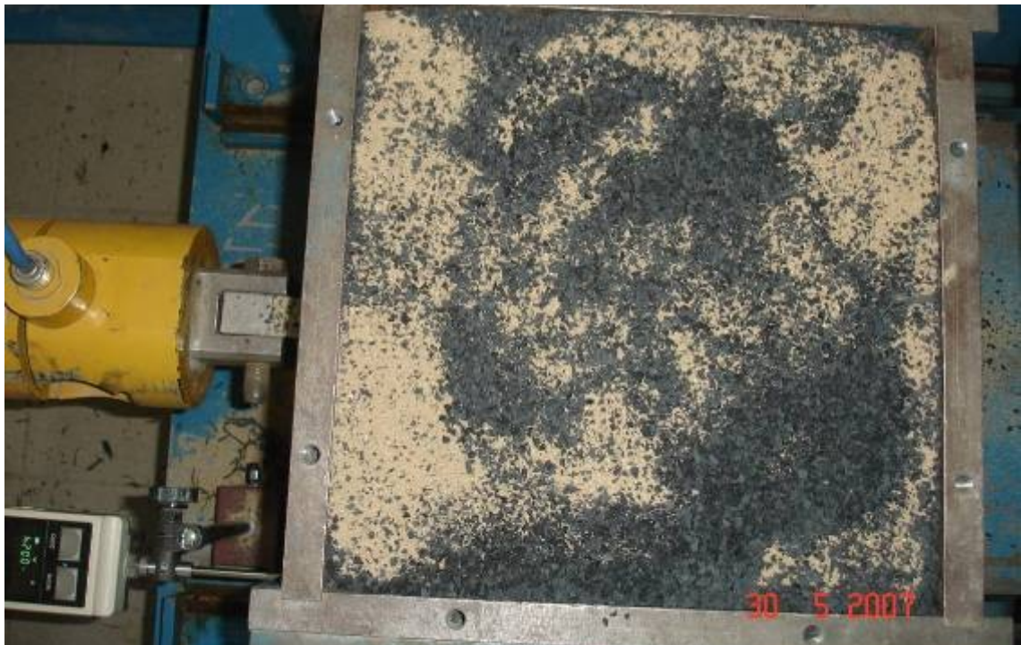
Figure 5.33. 20 per cent Tire crumb placed in the shear box
