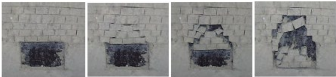
Figure 2.6. Studies of tunnel structure with base friction apparatus at TU Graz, Goricki (1999)
