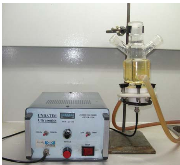
Figure 4.3. Photographic view of US2 (300 kHz plate type reactor).
