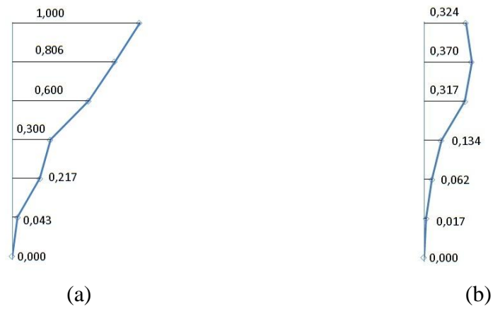
Figure 4.28. Second Mode Shape Amplitudes Before Strengthening: (a) E-W Direction, (b) N-S Direction.
