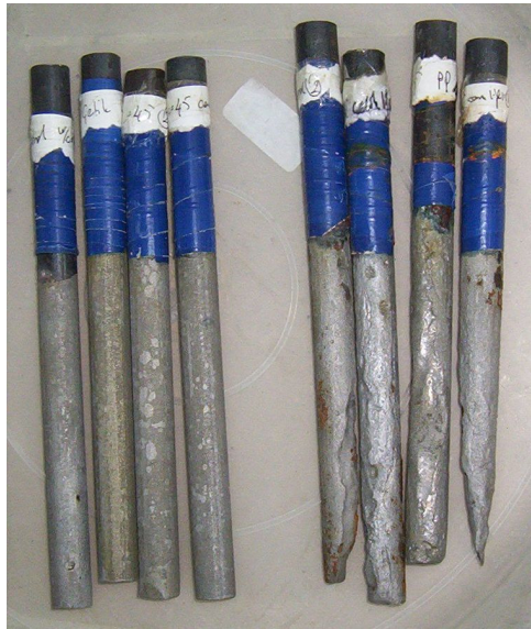
Figure C.2. Corrosion Damage. Steel bars after cleaning. Obtained from control concrete, SFRC, PFRC and GFRC from left to right (a) at first crack and (b) at the end of accelerated corrosion test
