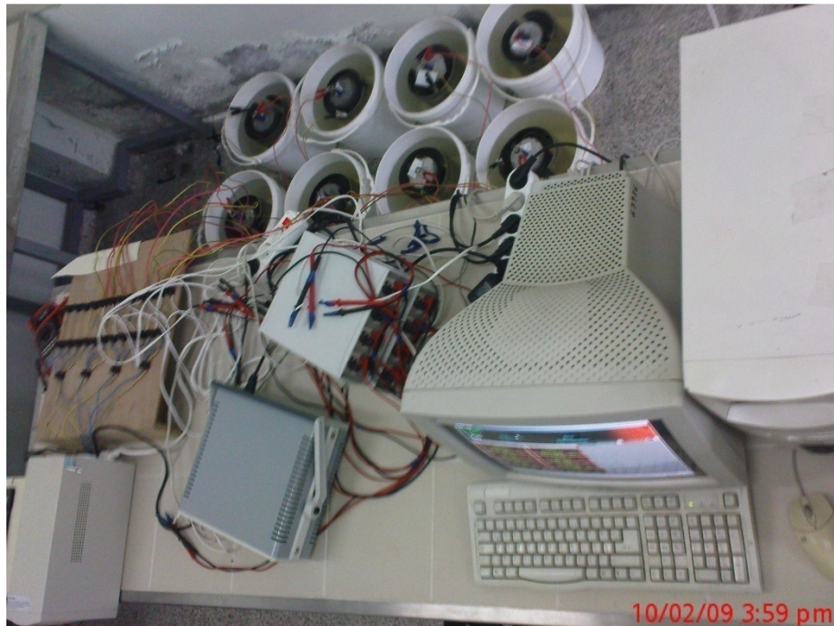
Figures A.1, A.2. Actual Setup of Accelerated Corrosion Test
