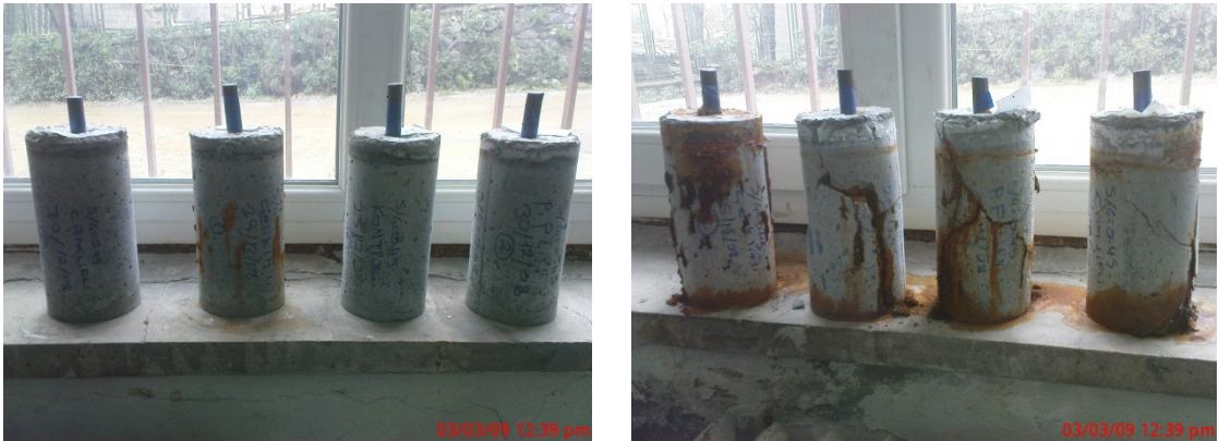
Figure C.1. Specimens at first crack (left); at the end of experiment (right)
