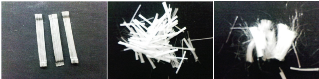
Figure 4.1. (a) Steel fibers, (b) Glass fibers and (c) Polypropylene fibers
