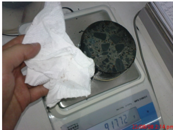
Figure A.4. Sorptivity Test Procedure. Removal of excess water; Weighing of specimen at specific time intervals
