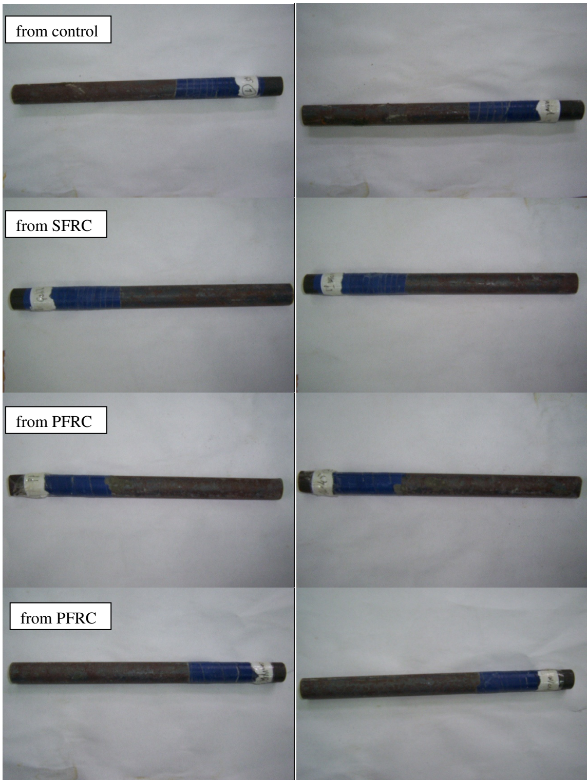
Figure 5.9. Pictures of removed steel bars before cleaning (pictures from opposite sides)
