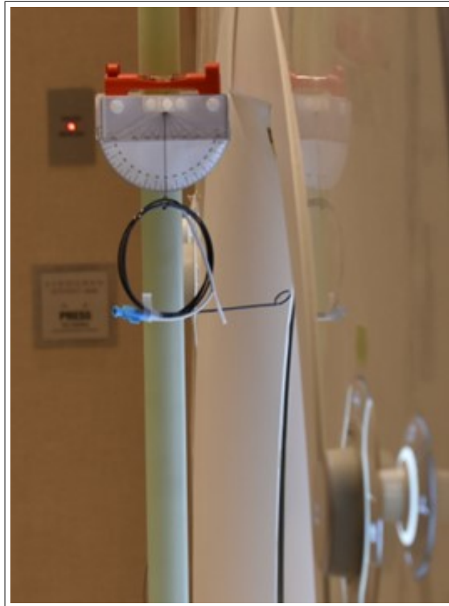
Figure 4.5 Magnetically induced force measurement test setup.
