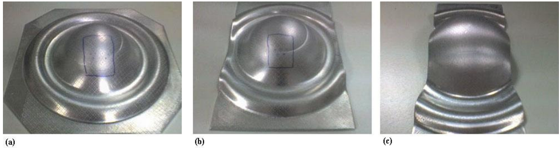
Figure 3.10. Three types of specimens used in the dome stretch test. (a) 110x110 mm, (b) 110x75 mm and (c) 110x50 mm
