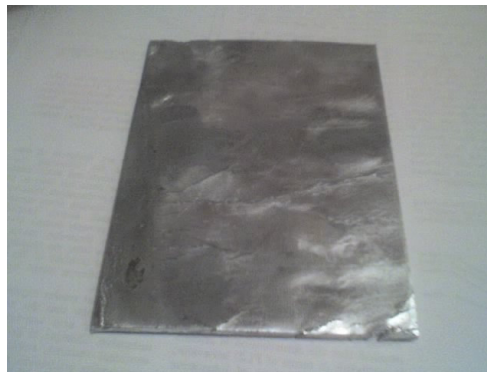
Figure 3.13. As-cast, 1.5 mm strip cast with the prototype twin-roll caster
