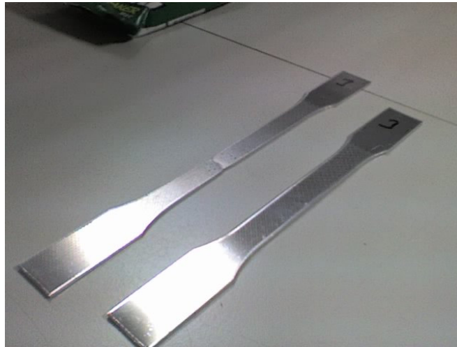
Figure 3.6. Electrochemically etched uniaxial tensile test specimens
