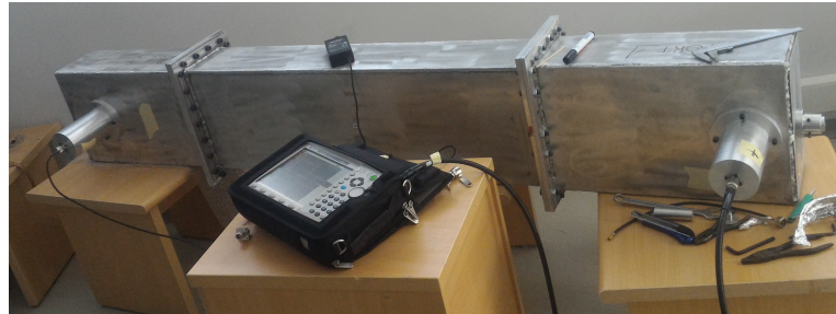
(a) Picture of the setup with the two converters including a 1 m waveguide.
