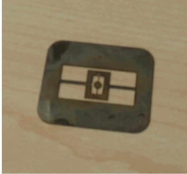
Figure 6.26. Photograph of the design with sub-arms and pair of outer flexures.
