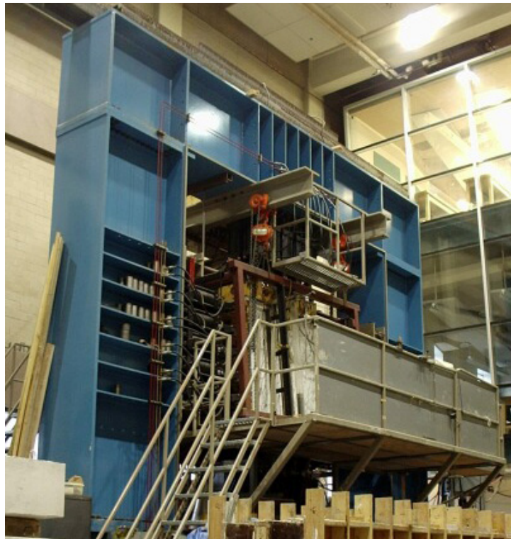
Figure 4.2. Shell Element Tester (University of Toronto)
