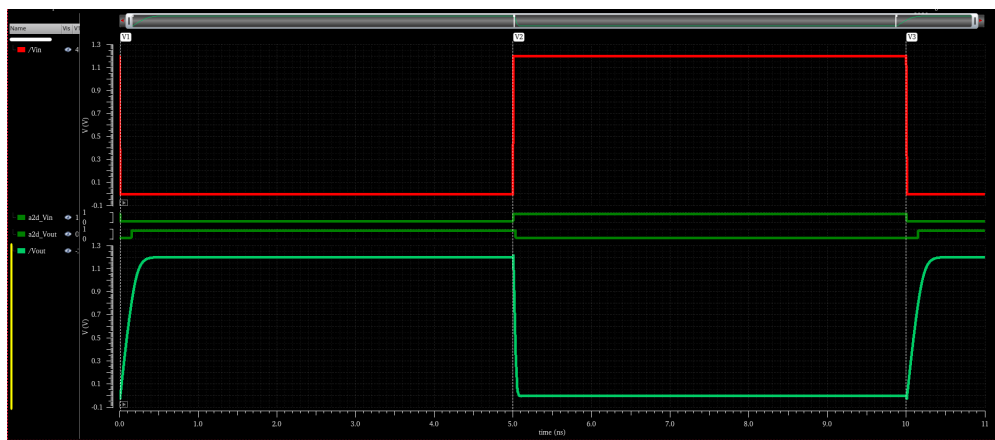
Figure 3.12. Example simulation result to illustrate rise-time, and fall-time effect.
