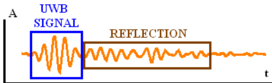
Figure 4.1. Reflections on a wideband signal.
