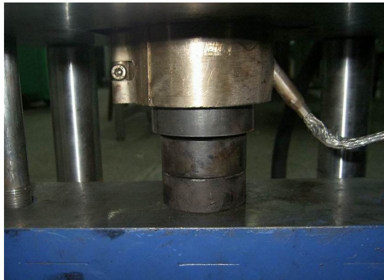
Figure 4.8. Closing the bottom hole of the die
