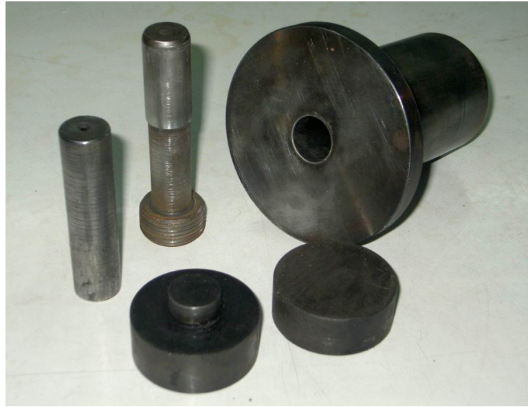
Figure 4.7. Die used to produce the specimens
