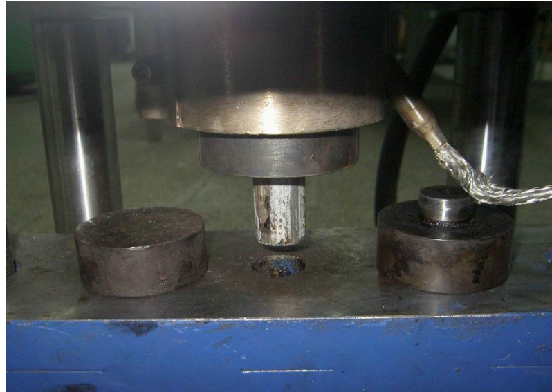
Figure 4.12. Removal of the sample from the die
