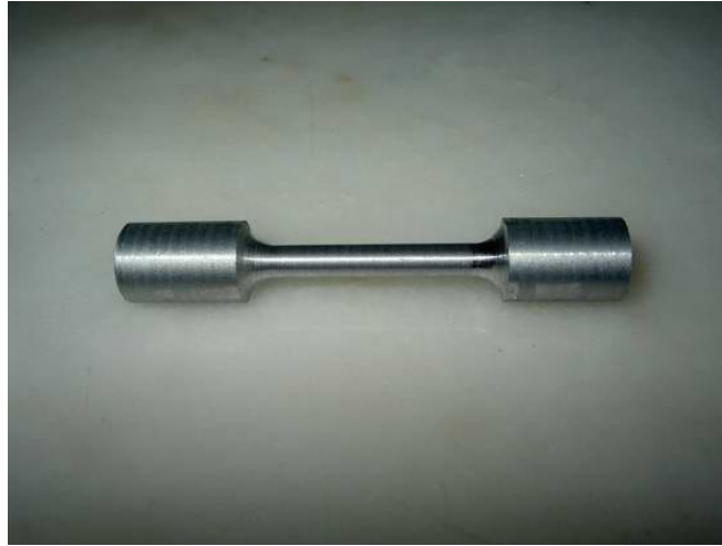
Figure 4.15. Image of the tensile test specimen
