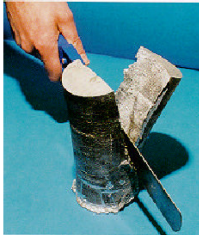
Figure 1.2. Cutting reheated billet with a spatula [3]
