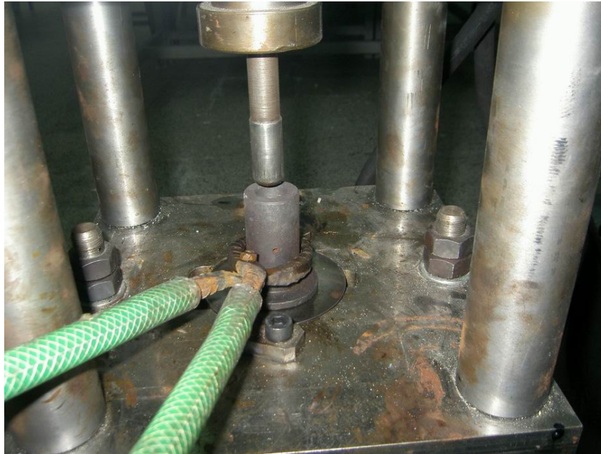
Figure 4.11. Transferring the heated billet to the die cavity
