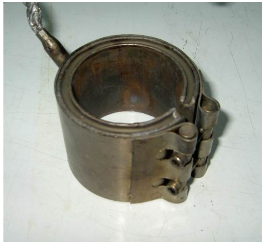
Figure 4.5. Ring heater used for pre-heating the die
