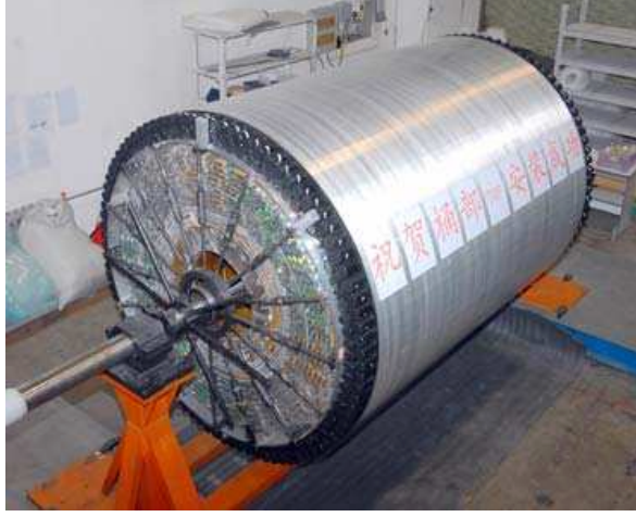
Figure 3.6. Two layers of barrel TOF counters taped to the outside of the MDC prior to the insertion into the electromagnetic calorimeter. The radius of the TOF counters is 870 mm [33].
