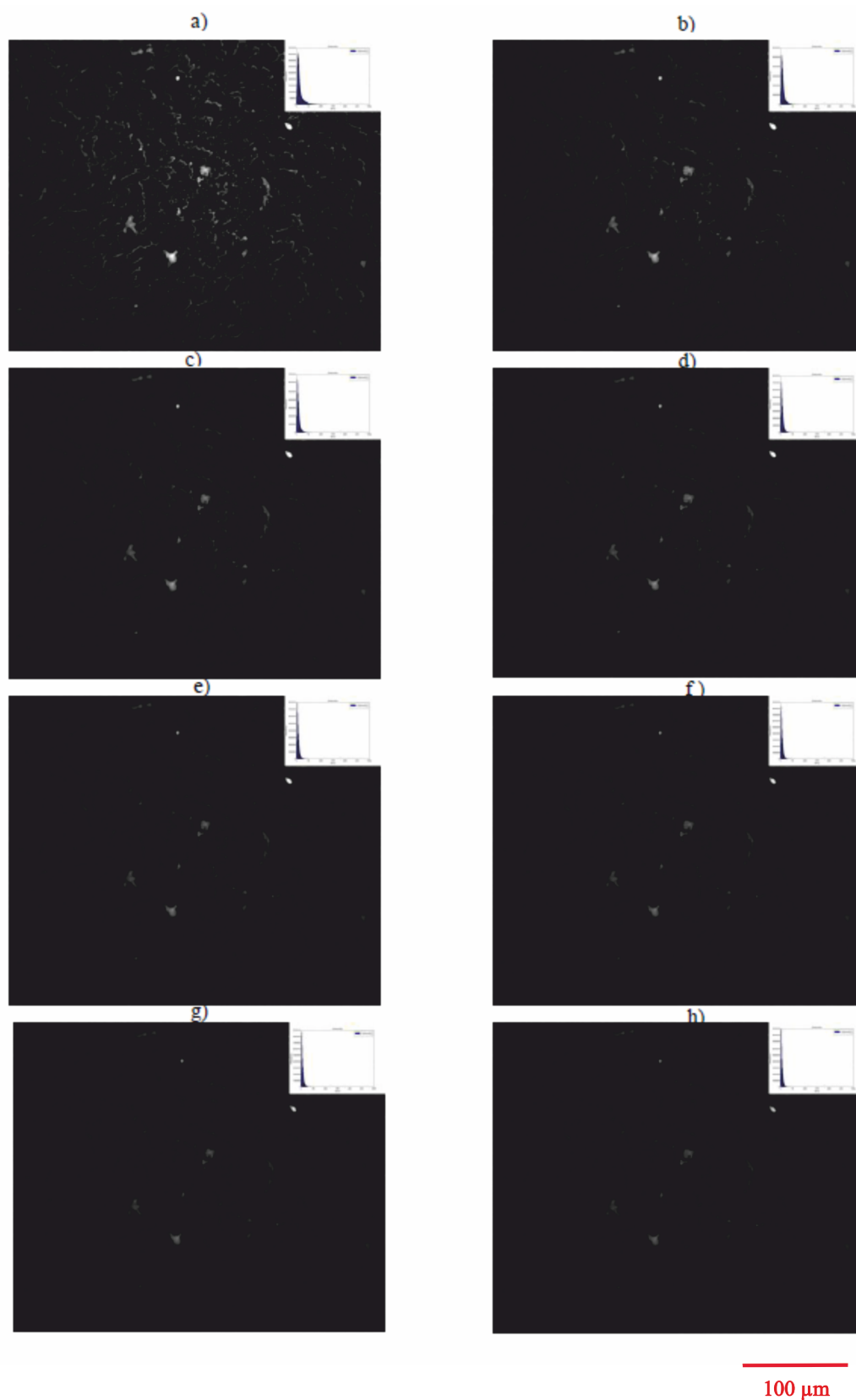
Figure 4.11. Photobleaching pace on fluorescent patterned sample surface. The images from (a) to (h) are taken in 10 seconds intervals.
