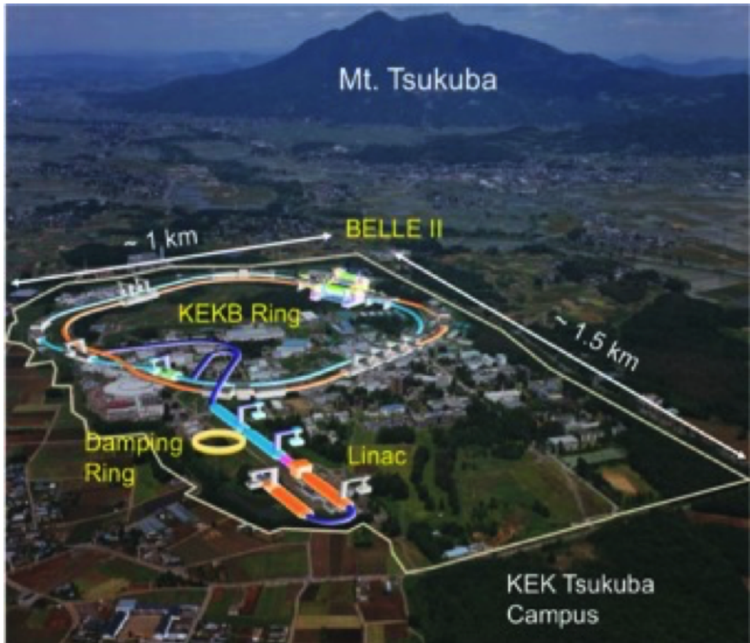
Figure 8.1. SuperKEKB layout. The J-shaped linac has a branching point for the positron damping ring. The injector linac provides e^- and e^+ beam with asymmetric bunch charge and energy to the collider with two rings.
