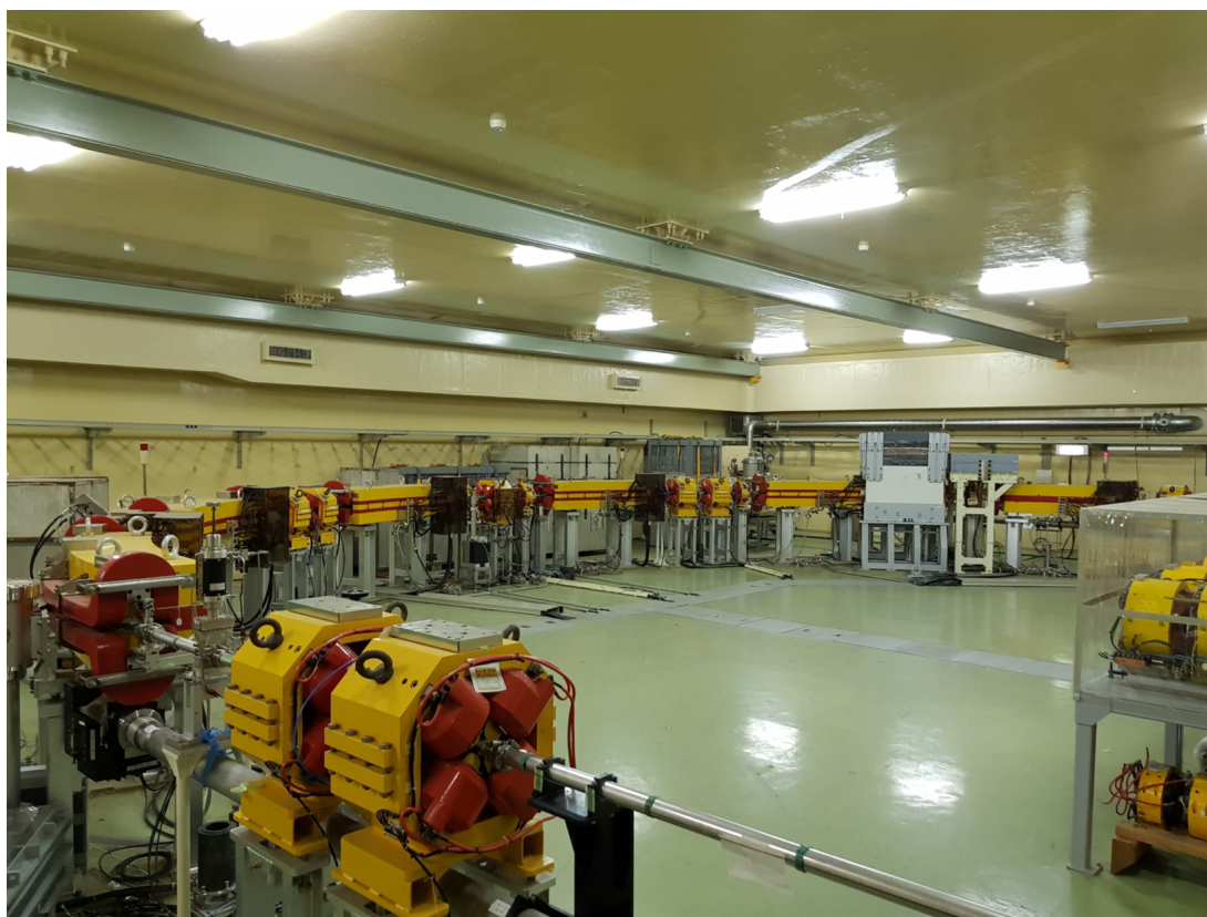
Figure 8.26. KEK 180° bend isochronous achromat which was built to bridge the extension to the old linac in parallel. Thus, the linac has become J-shaped.
