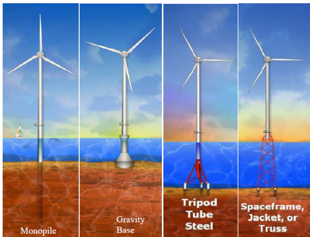
Figure 1.8. Shallow and deep-water foundation technologies [23]
