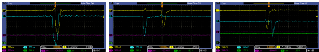
Figure 3.29: The screen-shot of the oscilloscope for the signals of the cosmic particles. Blue and yellow: readout from either end of the detector. Green: HV applied (scaled by a factor of 1000)
