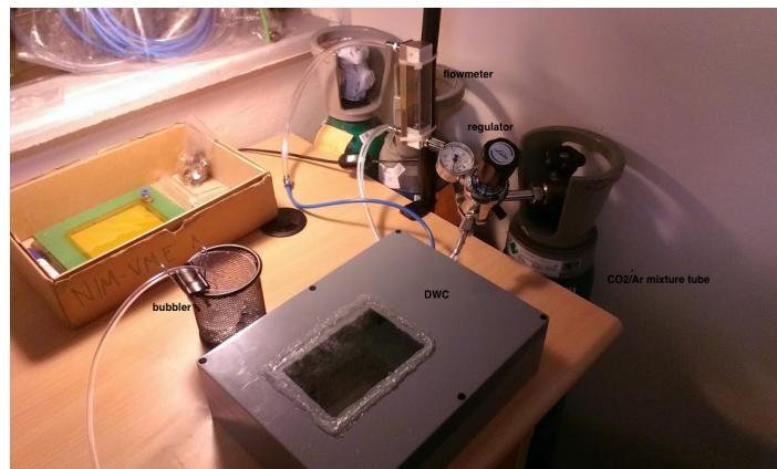
Figure 3.24: The gas system connected to the DWC
