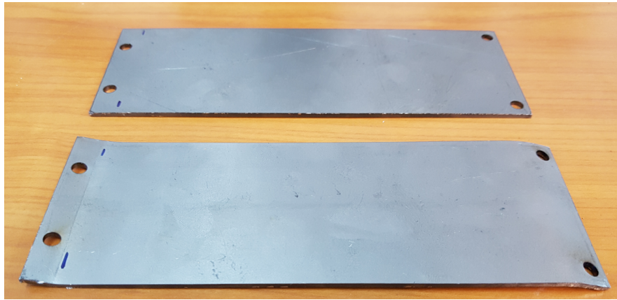
Figure 5.13. 2 mm plates before and after bending the edges.
