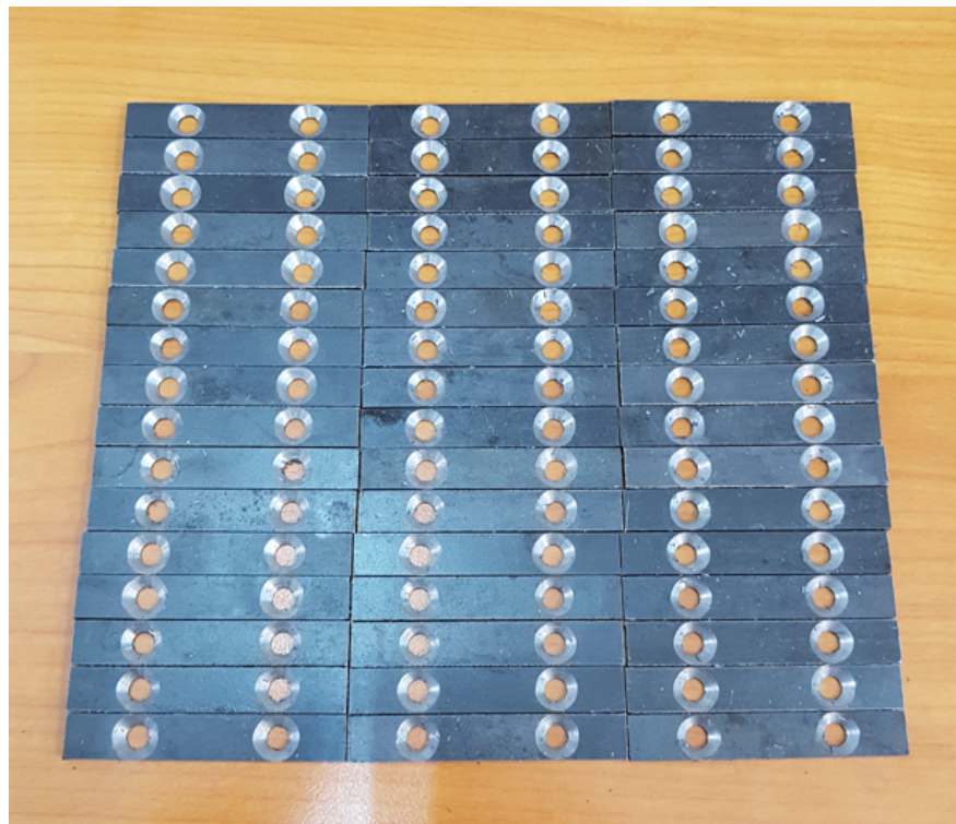
Figure 5.22. 48 pieces of fixing plate with 32 mm hole separation.
