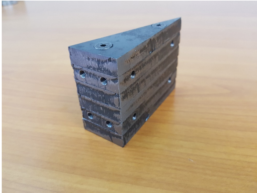
Figure 5.3. Six pieces of 10mm triangles are bolted together. The triangular block is tapped at 8 different points to enable attachment to the wall plate and bottom plate.
