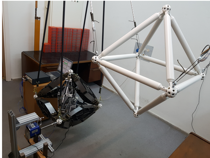
Figure 6.1. Test benches of octahedron structures made up of inertial amplification mechanisms (left) and steel rods (right).
