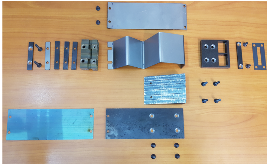
Figure 5.30. Short wall assembly components before assembly.
