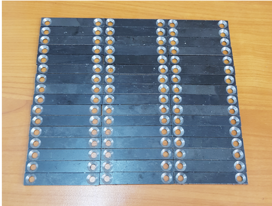
Figure 5.23. 48 pieces of fixing plate with 52 mm hole separation.
