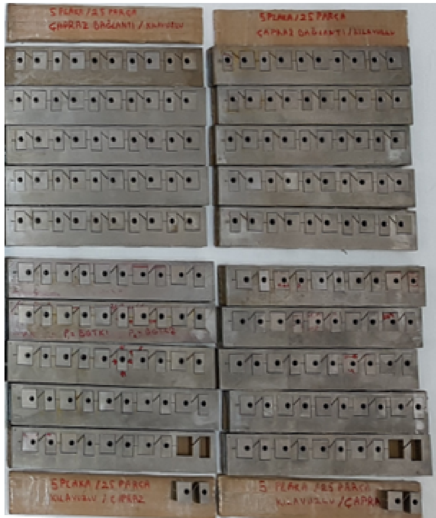
Figure 5.15. Cross flexures cut from 10 mm plate by wire EDM.
