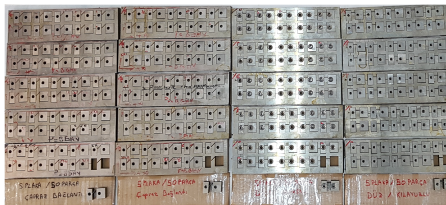
Figure 5.16. Cross and straight flexures cut from 10 mm plate by wire EDM.
