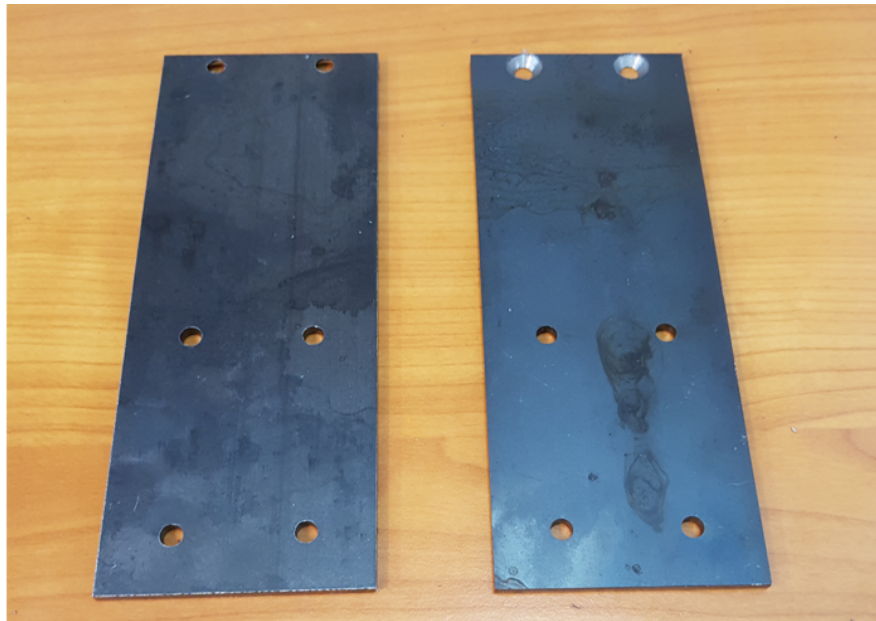
Figure 5.11. 3 mm plates countersunk to be connected to cross flexures.
