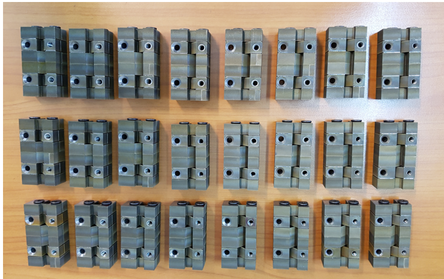
Figure 5.20. 24 bottom flexure assembly.
