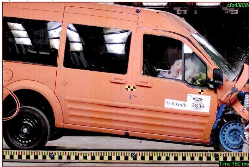
Figure 5.24. Vehicle deformation during 56 km/h offset impact test, (t=150ms)
