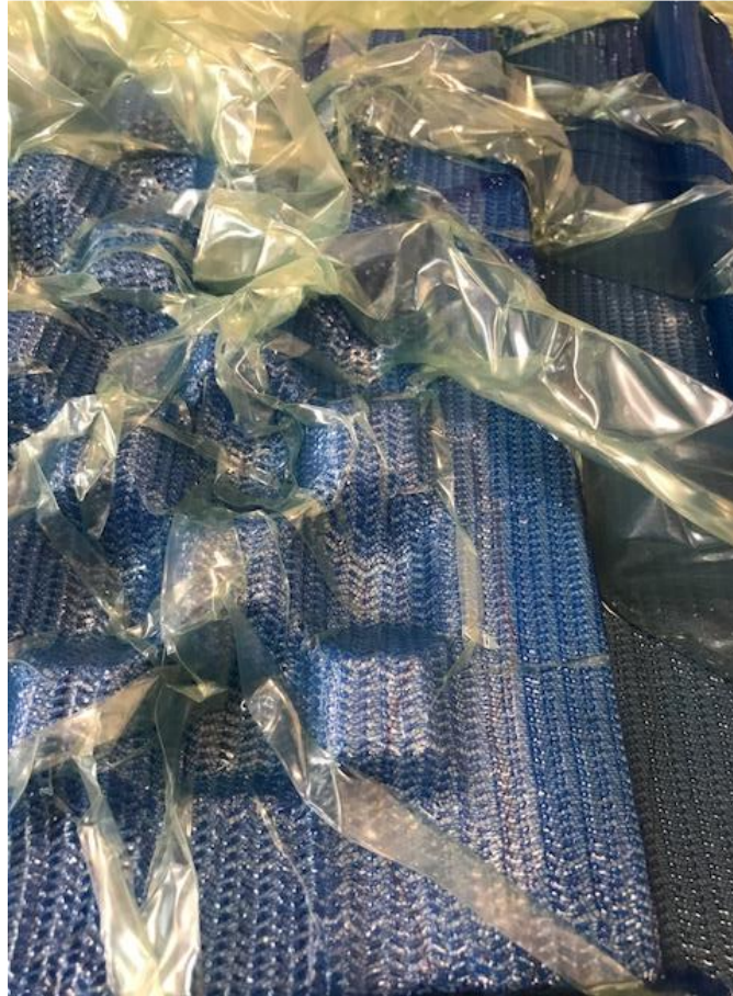
Figure 3.12. Resin impregnation to the core section.
