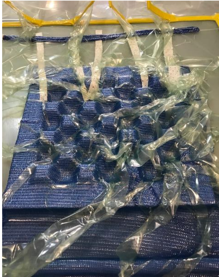
Figure 3.11. Core section setup under vacuum pressure.
