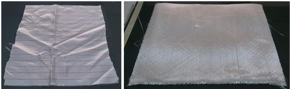
Figure 3.7. (a) Peel ply, and (b) E-glass fiber reinforcement.
