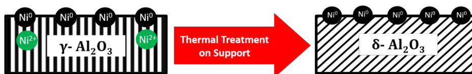
Figure 4.29. Schematic representation of the effect of thermal treatment on nickel dispersion.
