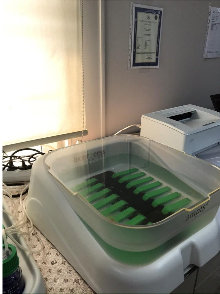
Figure B.9. AMPTS in the BMP test.
