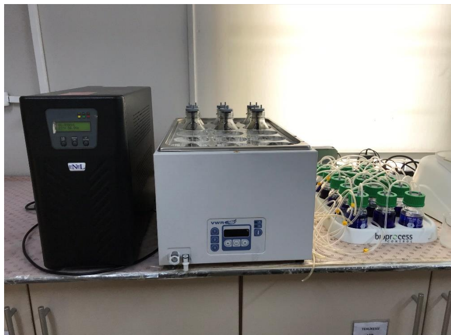
Figure B.6. BMP test equipment.
