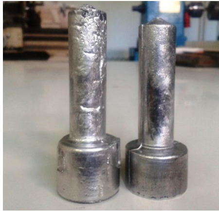
Figure 3.36. As cast specimens not-squeezed (left) and squeezed (right).
