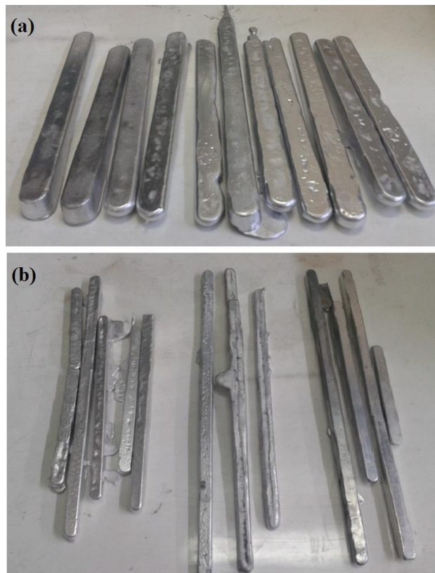
Figure 3.7. Samples of (a) Master ingot 10 % BN-Al (b) master ingot 10 % B_4C -Al.
