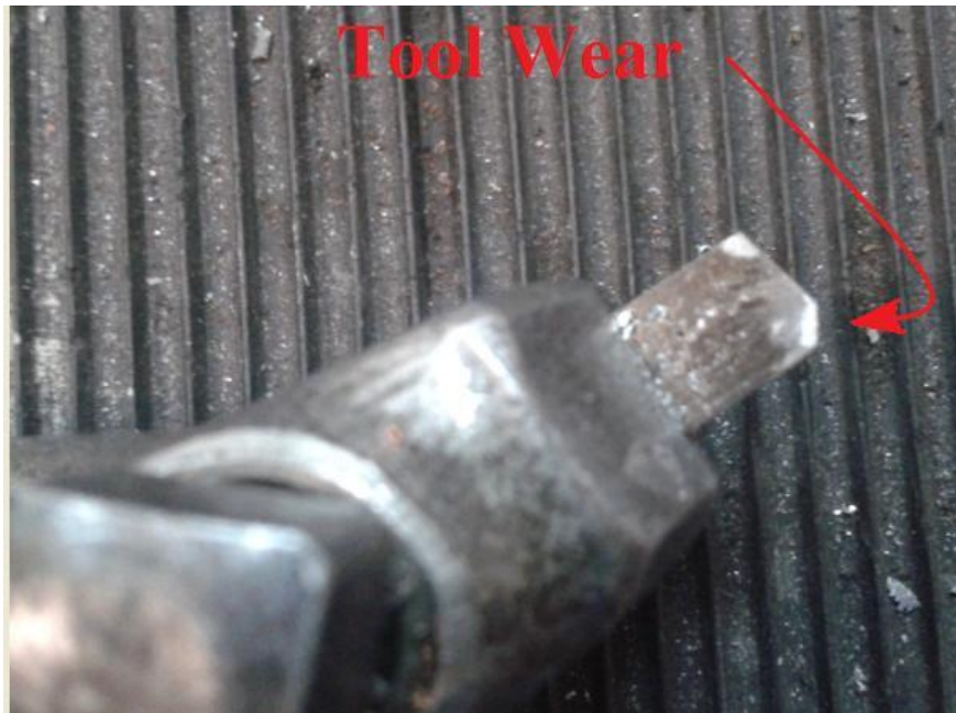
Figure 3.20. Tool wear (HSS) after one pass on a sample containing 5 % boron carbide.
