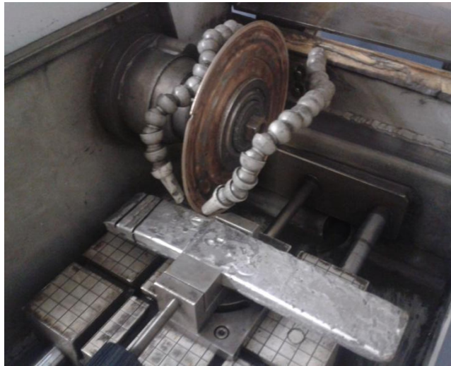
Figure 3.17. Cutting master ingot 10 % B_4C -Al with diamond cutting tool.
