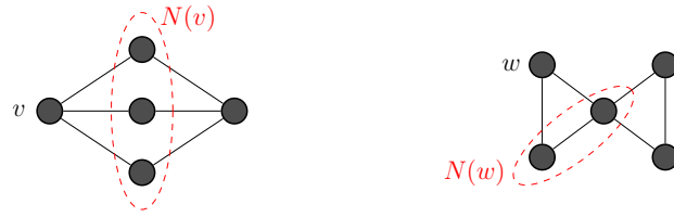
Figure 2.2. Two graphs on which neighborhoods N(v) and N(w) of vertices v and w are shown in dashed ellipses, where d(v) = 3 and d(w) = 2 .
