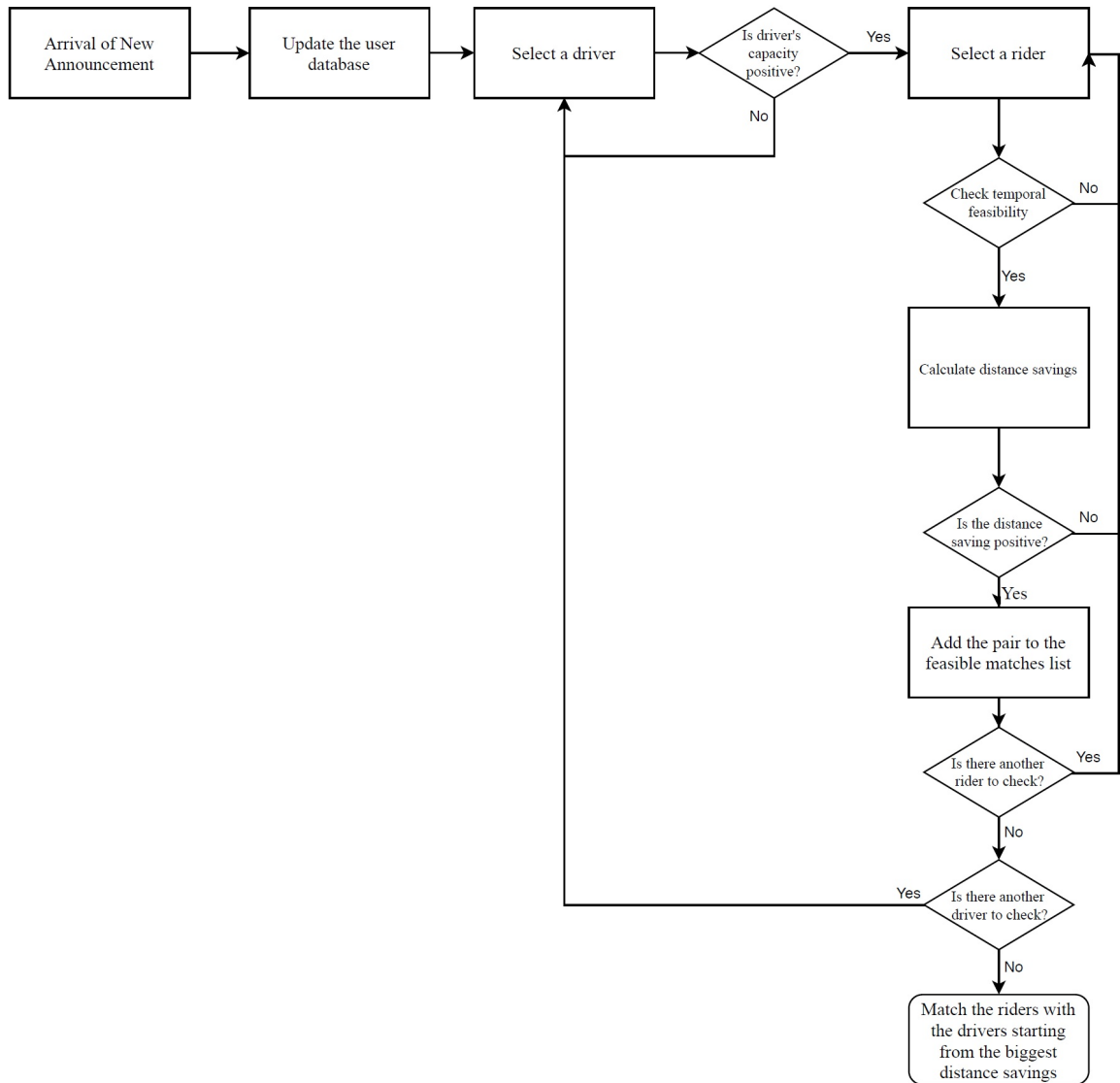
Figure 5.2. Flowchart of the weighted bipartite ride-matching algorithm.
