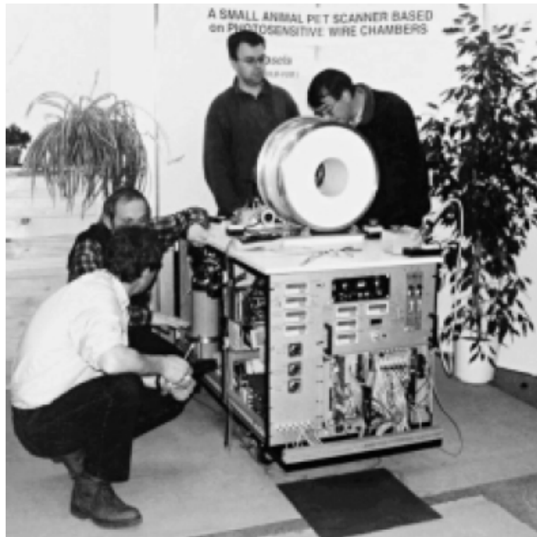
Figure 4.17: The TMAE-PET prototype based on TMAE vapour and Multi-Wire gas avalanche chamber [78].
