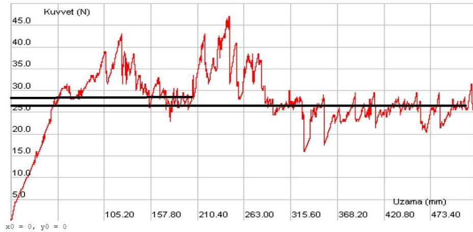
Figure 3.11. Interpolation of interlaminar adhesion test graph.
